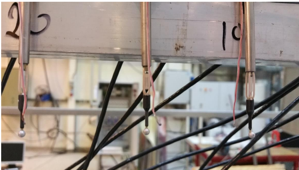
Figure 15: Sensors. Ball shape is velocity and other is temperature
