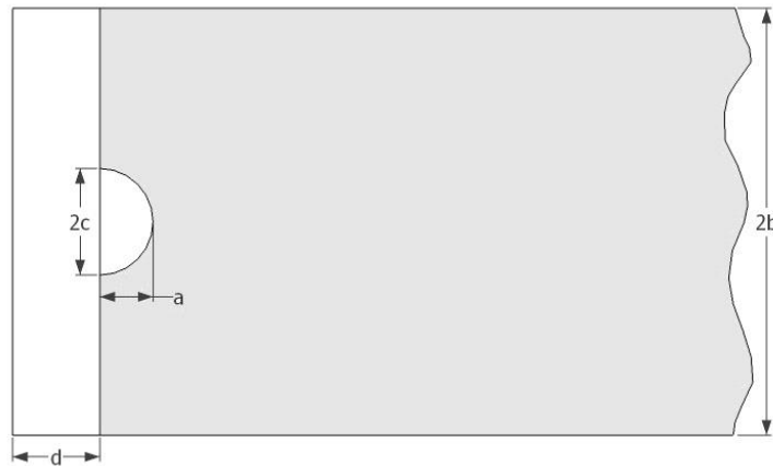
Figure 42 Crack plane for notched plate
