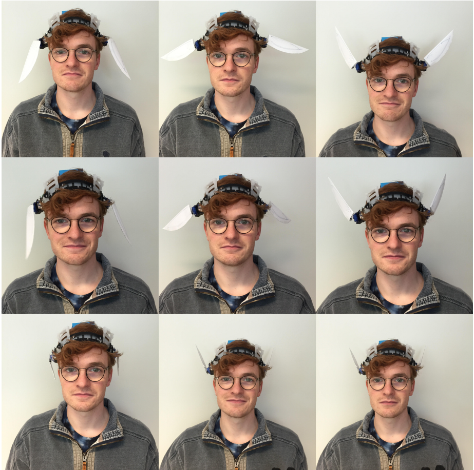
Figure 6.8: Collage of different ear positions. The x-axis goes from minimum to maximum rotation, and the y-axis goes from minimum to maximum tilt.
