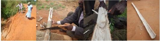
Figure 32 Sisal gutter - image sequence
