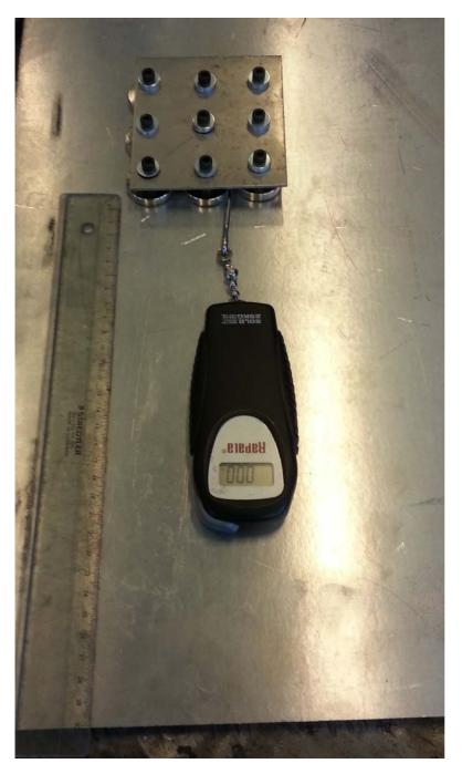
The same test was done on a welding table of steel to see what kind of force the magnets would generate against a steel plate. This is not eddy current working and the force will therefore not be affected by speed.
