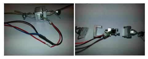
Figure 15: Homemade load cell, exploded view to the right (see appendix H)
