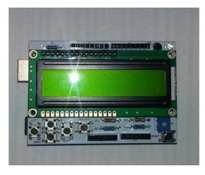
Figure 16: The LCD breakout board
