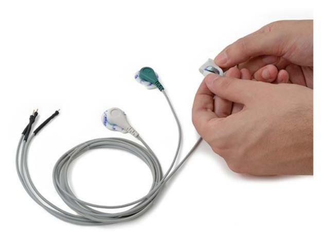
This sensor use disposable pre-gelled electrodes.
