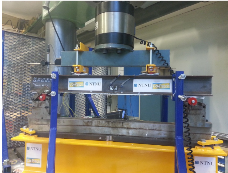
Figure 22 – Setup of four point bending test
