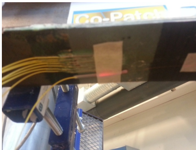
Figure 37 – Testing with laser to check if the fiber is broken
