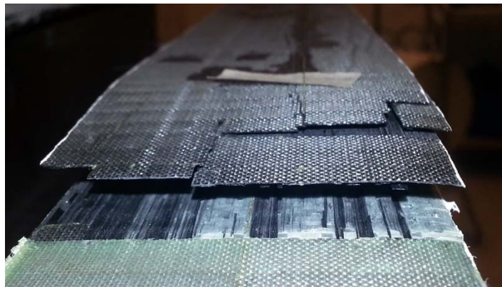
Figure 56 – Delamination in different layers, beam #23
