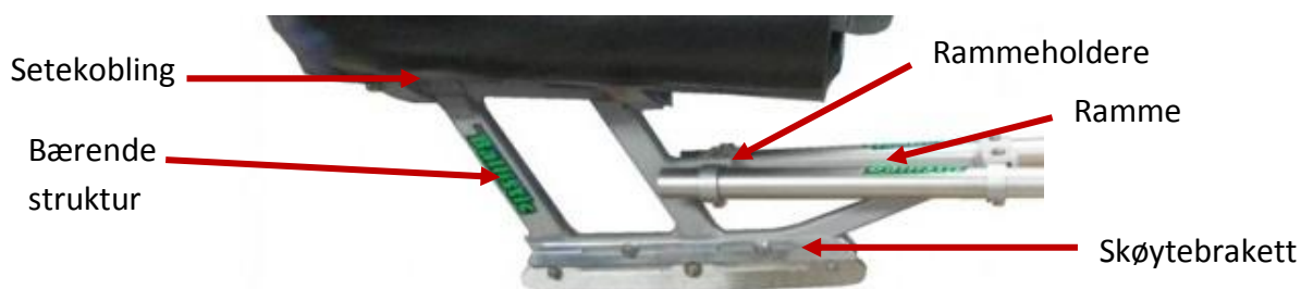
Figur 30 - Deler i understellet til Ballistic ( uniqueinventions.com/ballistic )
