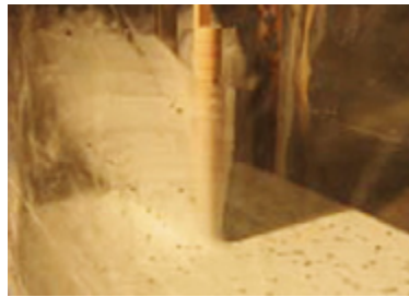
Figure 1.7: Fan-shaped stream of granular material around a slender cylindrical obstacle. From: Hauksson et al. (2007) .
