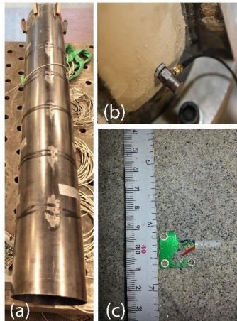
Figure 7-5. Instrumentation: (a) strain gauges mounted on the lower part of the pile; (b) accelerometer mounted just above the connection flange; and (c) accelerometer to be buried in the sand
