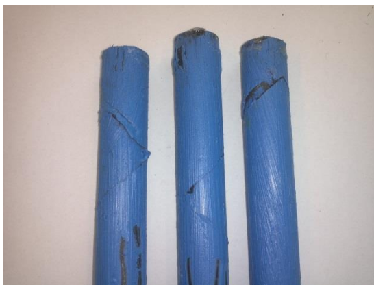
Figure 4-9: Failed [\pm 45^\circ] samples after high pressure testing
