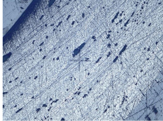
Figure 4-4: Microscopy of [\pm 45^\circ] samples, \theta -R plane cross section
