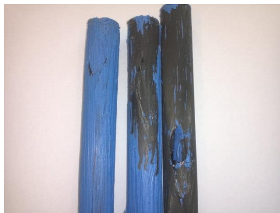
Figure 4-10: Failed [\pm 80^\circ, \pm 9^\circ] samples after high pressure testing
