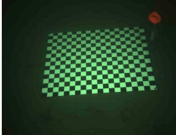
Figure 2.23: Checkerboard is used underwater to calibrate camera for distortion
