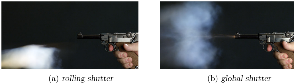
Figure 2.11: rolling compared to global shutter, courtesy of http://www.red.com/learn/red-101/global-rolling-shutter
