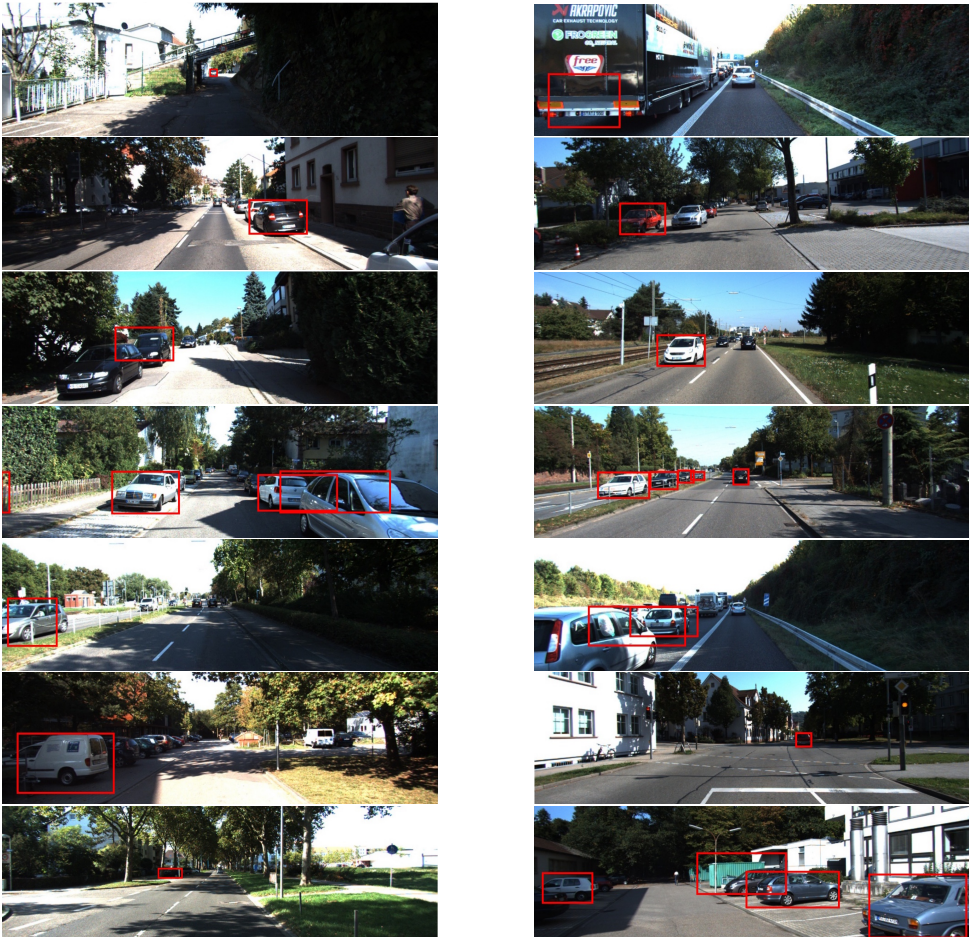
Figure A.1: Randomly sampled detections made by our best performing detector on KITTI Validation K-BG (t&o), from the KITTI Validation dataset.
