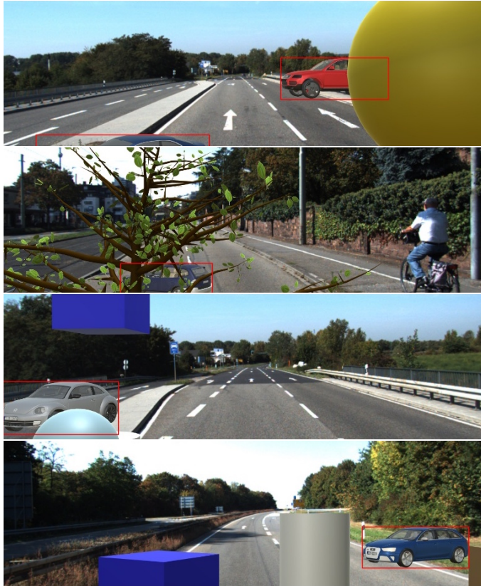
Figure 3.11: Dataset images with occlusion and truncation. Labels, highlighted in red, still outline the complete car shape within the bounds of the image.
