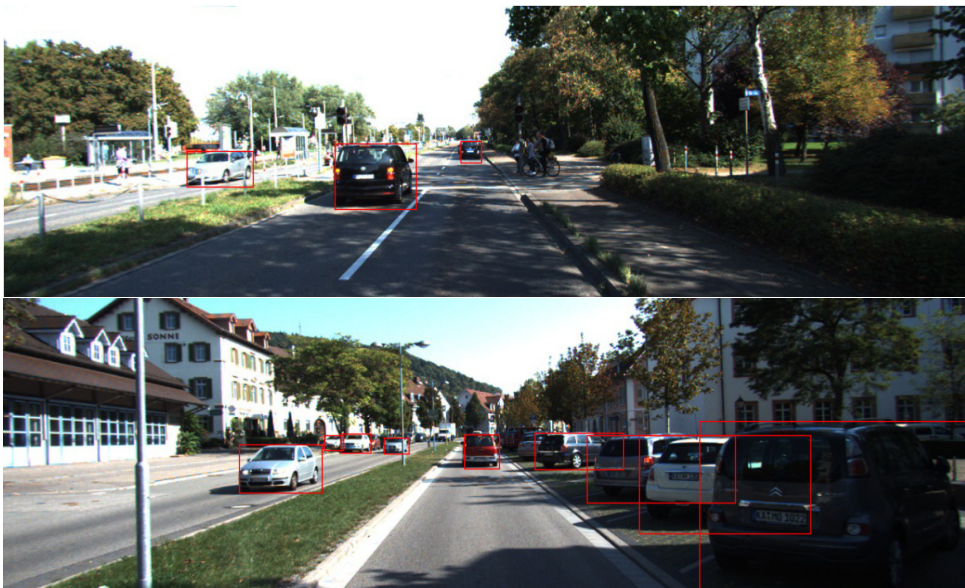
Figure 3.4: Example images from the KITTI dataset with ground truth bounding boxes for the car category overlaid
