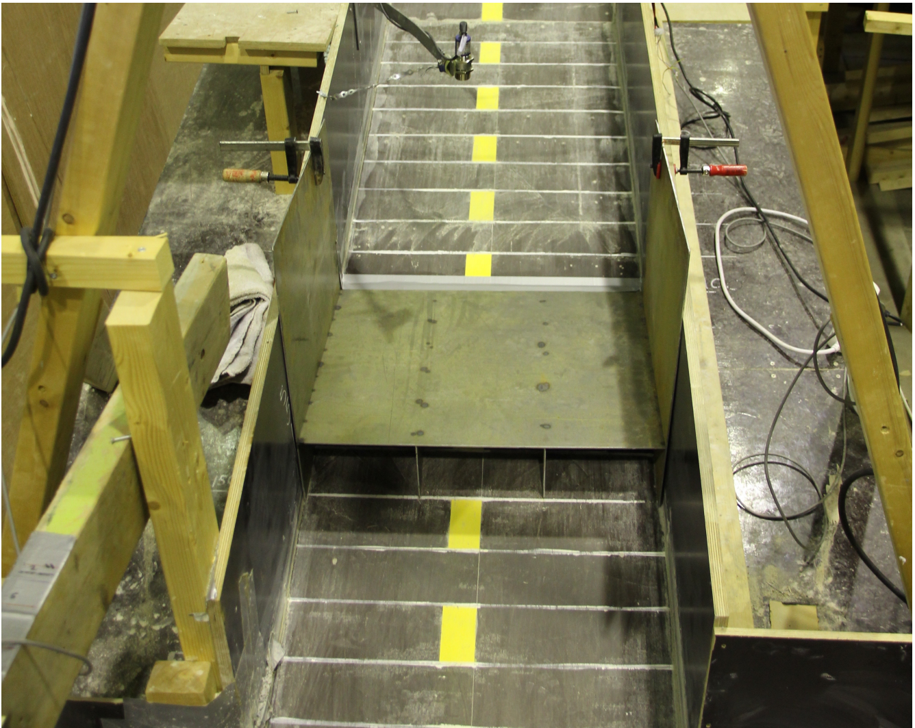
Figure 4.10: The 0.5 m long solid plate which represents the debris flow breaker with 0 mm opening width. Two clamps are used to keep the structure in place. Duct tape is also used to create a smooth transition from the channel and onto the solid plate.
