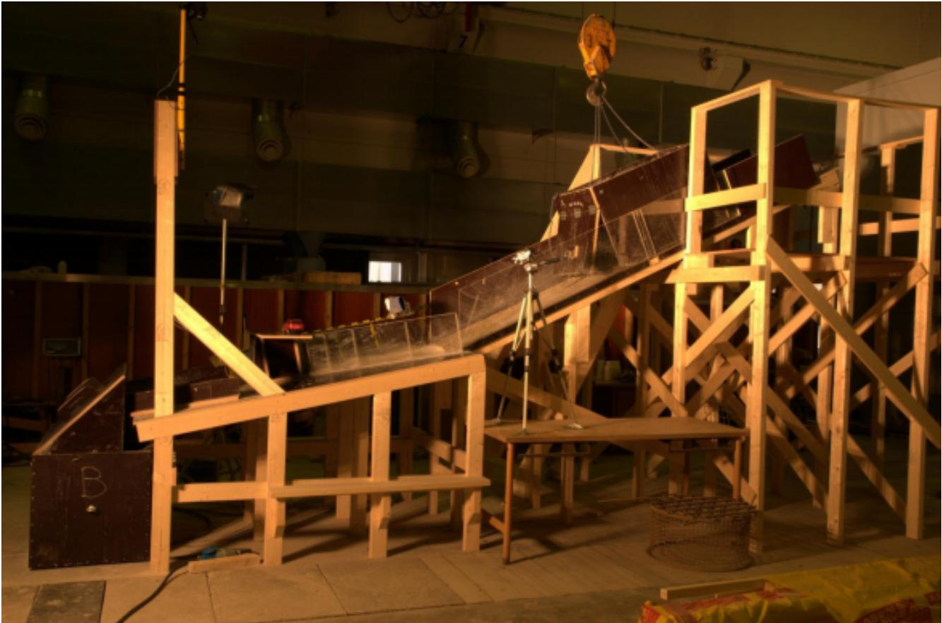
Figure 4.1: The debris flow model in 2009 when it was used to investigate the effect of channeling debris flows under a bridge by using deflection structures (Hiller and Jenssen, 2009).
