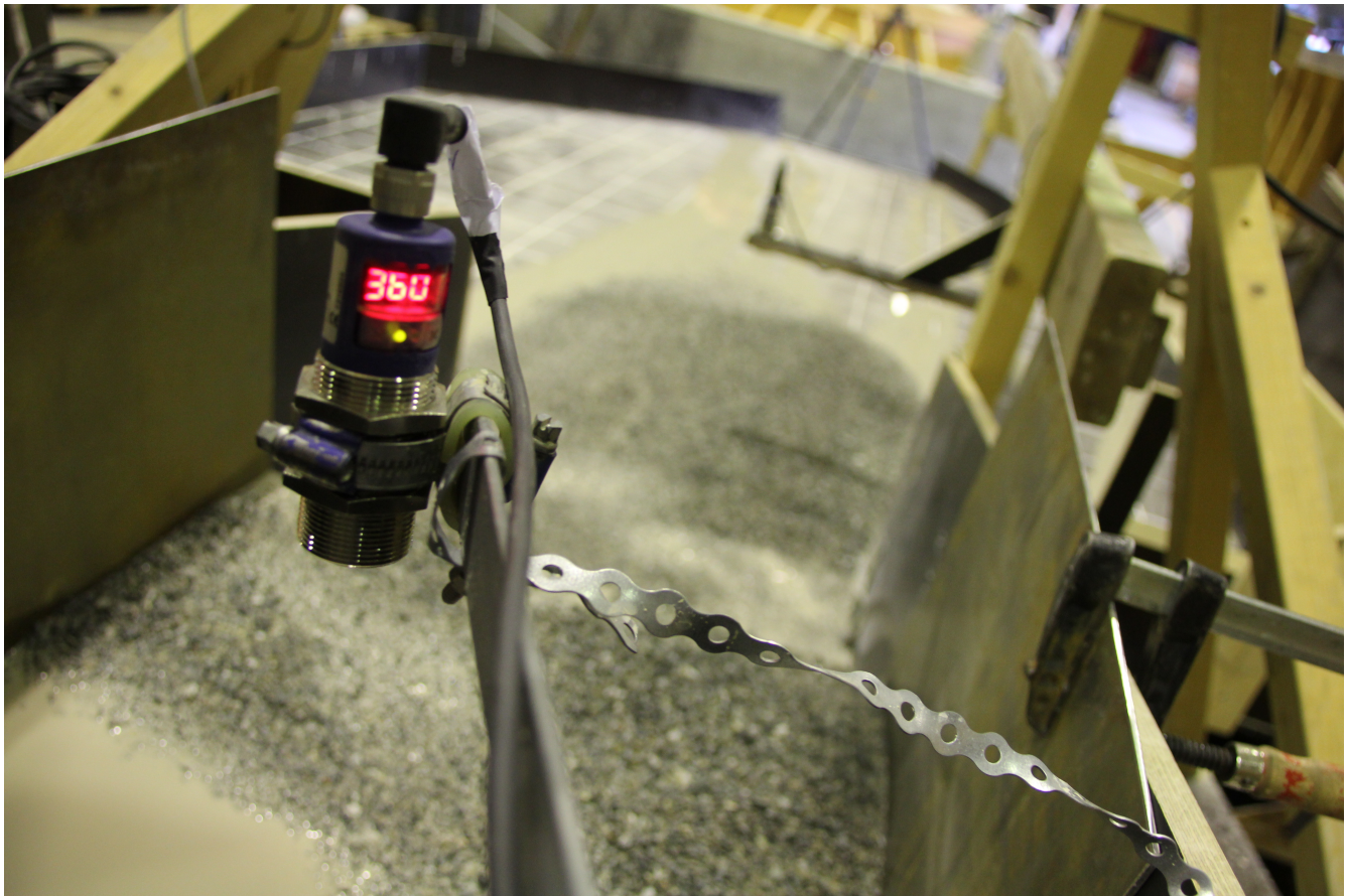
Figure 5.11: The display of the ultrasound sensor placed upstream of the debris flow breaker in the center of the channel at x = -115 .
