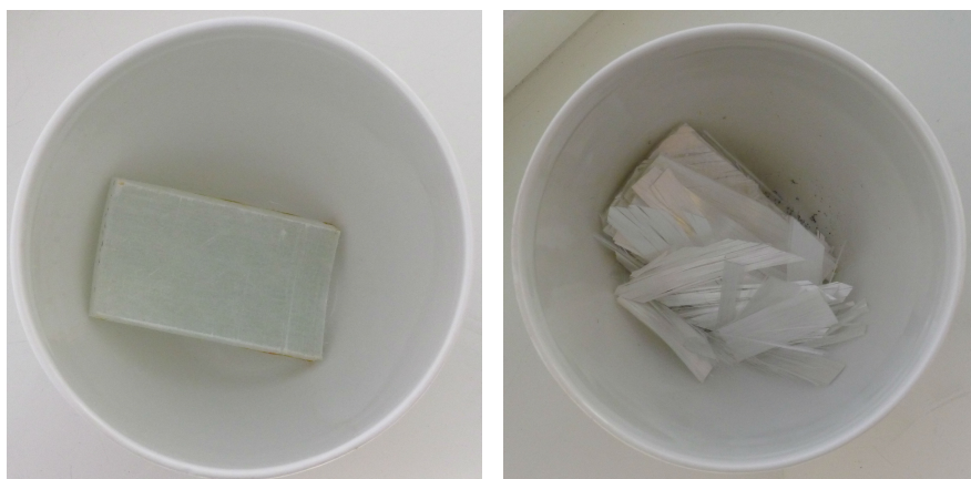
(A) Sample nr. 6 before burn off (B) Sample nr. 6 after burn off.
