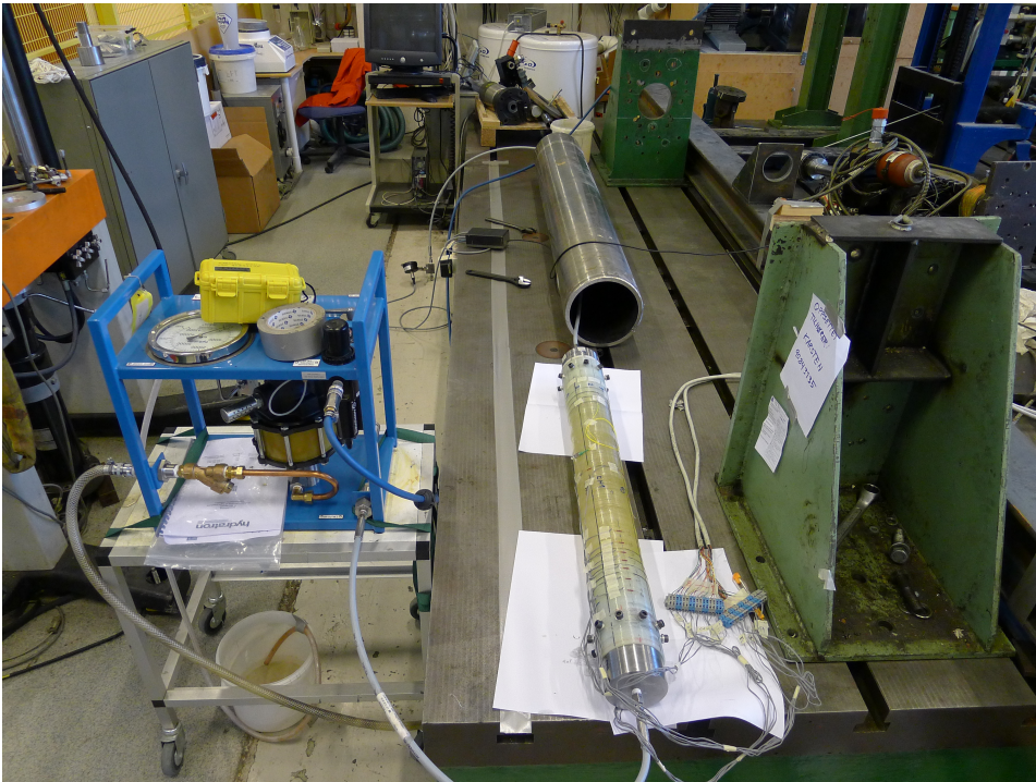
FIGURE 5.5: Pressure test setup.
