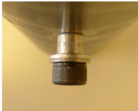
FIGURE 3.6: Bolt assembly. From the top: Hub, bushing, washers, screw head.
