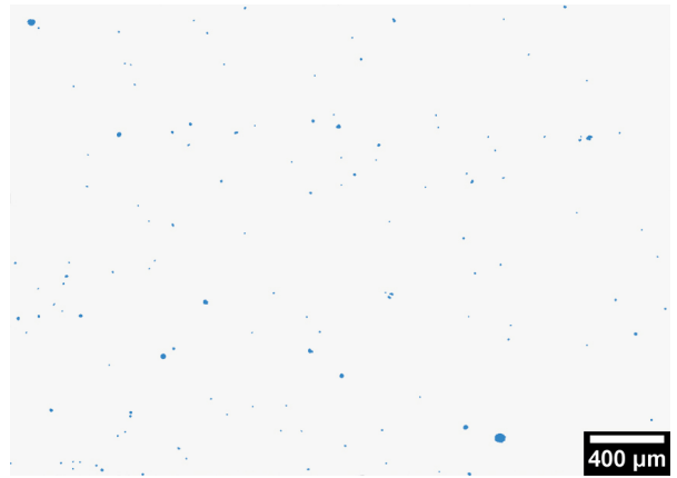
(b) Metallurgical pores.
