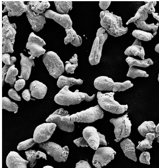
(a) AlSi10Mg low magnification.
