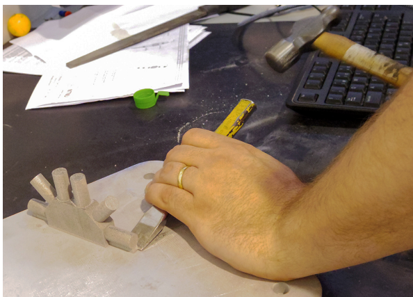
(a) Removal by chisel.
