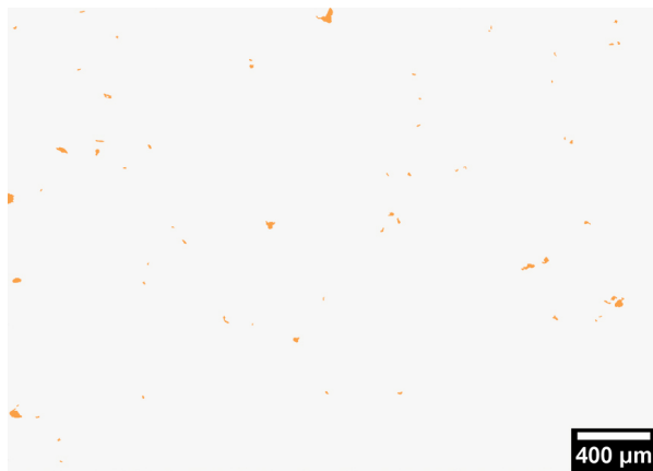
(c) Disrupted oxides.
