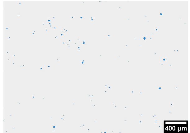
(b) Metallurgical pores.
