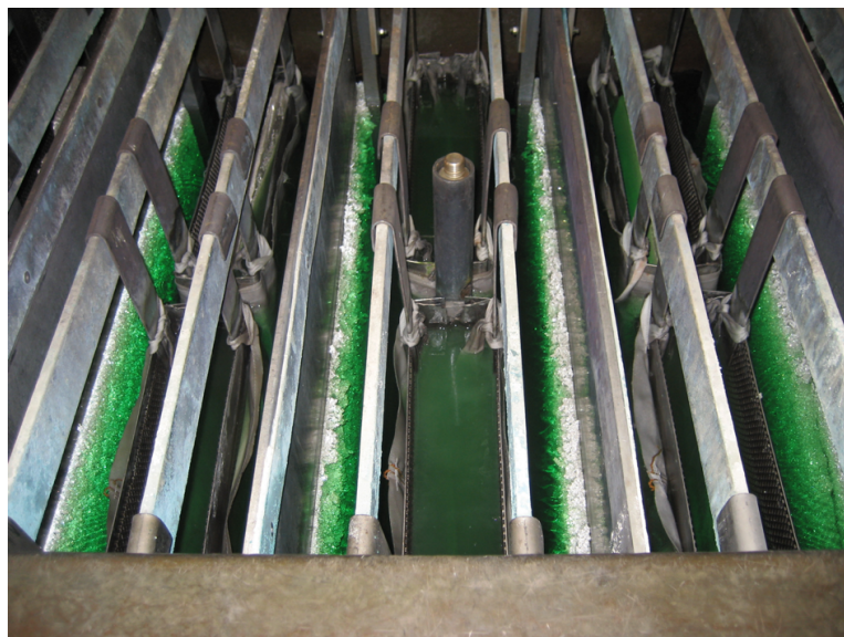
Figure 2.3 – Electrolysis cell for silver catalyst production, provided by K.A. Rasmussen.
