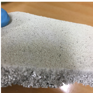
Figure 4.1 – Image of the plant exposed catalyst. Visual changes is apparent in the top layer of the silver catalyst.
