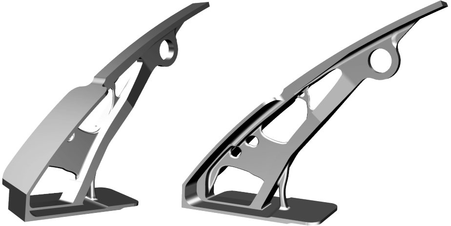
Figure 5.3: Door Connection Joint; Reengineered geometry from minimizing volume and constraining displacement
