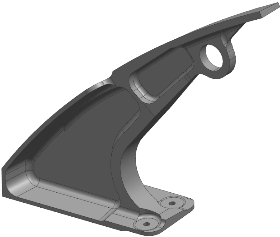
Figure 1.6: Door Connection Joint; Original CAD geometry
