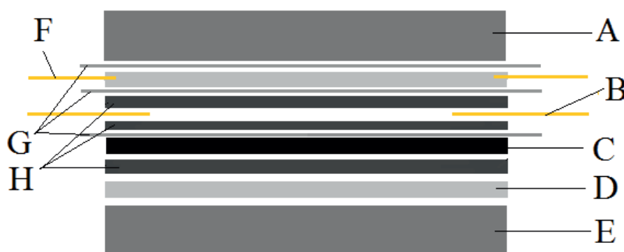
Figure 1: Setup for in situ measurements of ICR. A) Cathode housing. B) Gold wires placed in between sheets of GDL. C) MEA. D) Bipolar plate. E) Anode housing. F) Gold wires welded to bipolar plate. G) Gasket, preventing contact between gold wires and other electrically conducting parts of the fuel cell. H) GDL.
