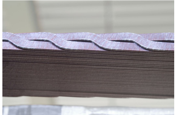
(b) Intertwining of a Roebel bar [8]
