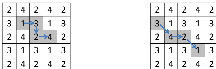
(a) A pseudo-pixel formed by rectangularly connected pixels (b) A pseudo-pixel formed by diagonally connected pixels
