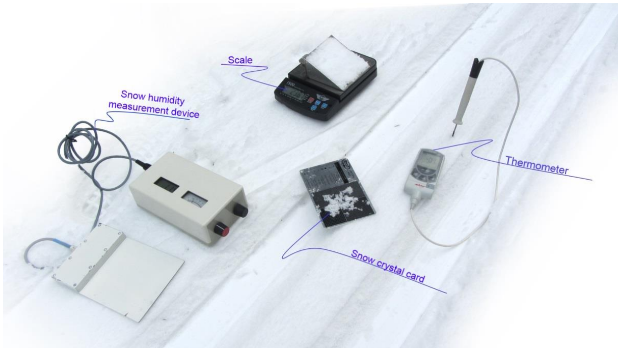
Figure 29 The equipment used to measure the weather and snow conditions during the field tests.
