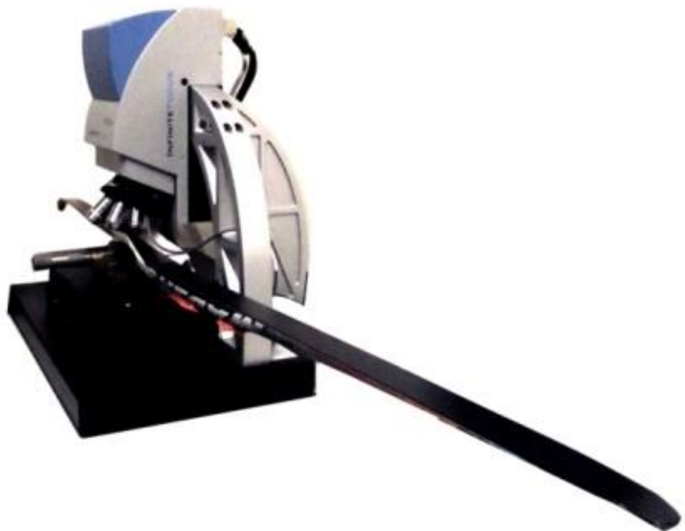
Figure 32 The confocal microscope is here used to find an approximate roughness on the ski bases used so the same grinding was used on all the material tested.
