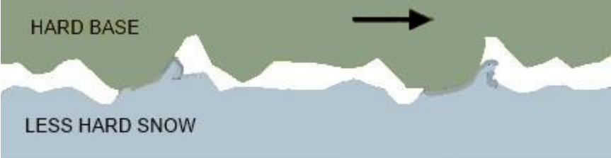
Figure 20 Adhesive ploughing, the hard base deforms the less hard snow and creates friction [37].
