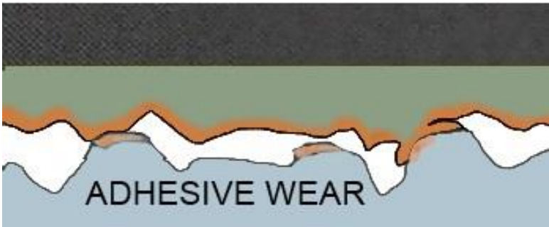
Figure 22 Adhesive wear, without a water layer material transfer from wax to snow may occur.
