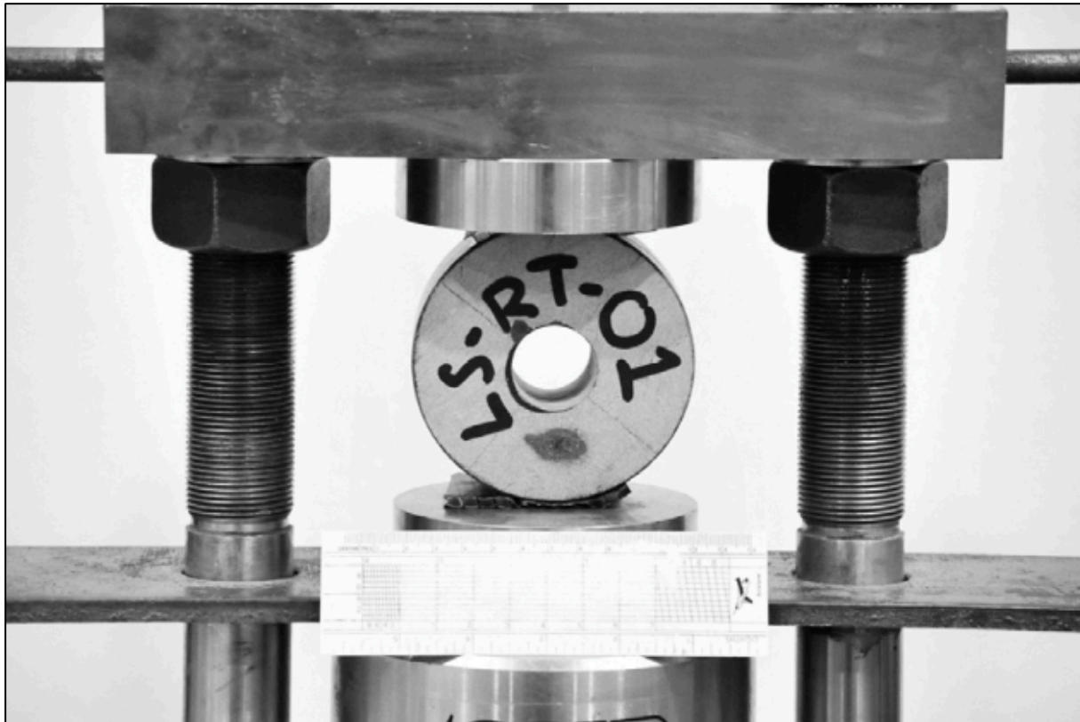
Figure 3-4: Setup for ring tension test (Klanphumeesri, 2010)
