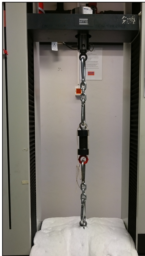
Figure 4-1: Experimental setup for the direct tensile strength test
