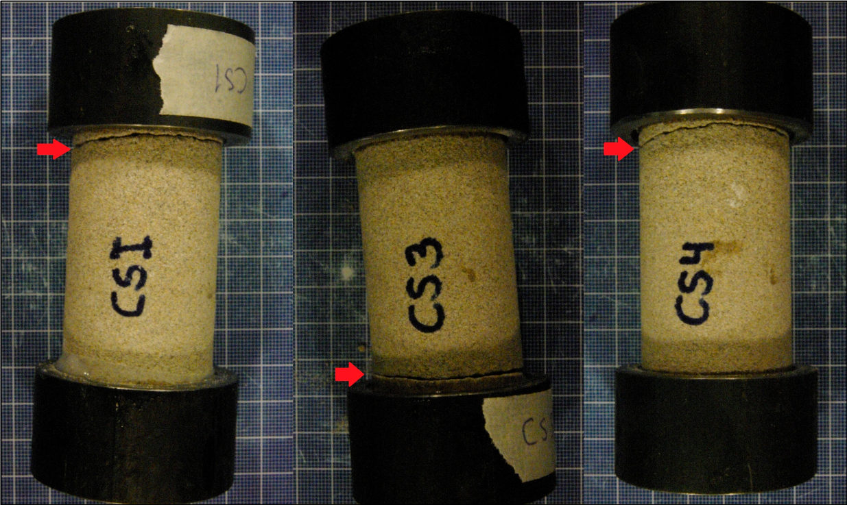
Figure D-8: Castlegate sandstone (diameter approximately 1.5") after testing
