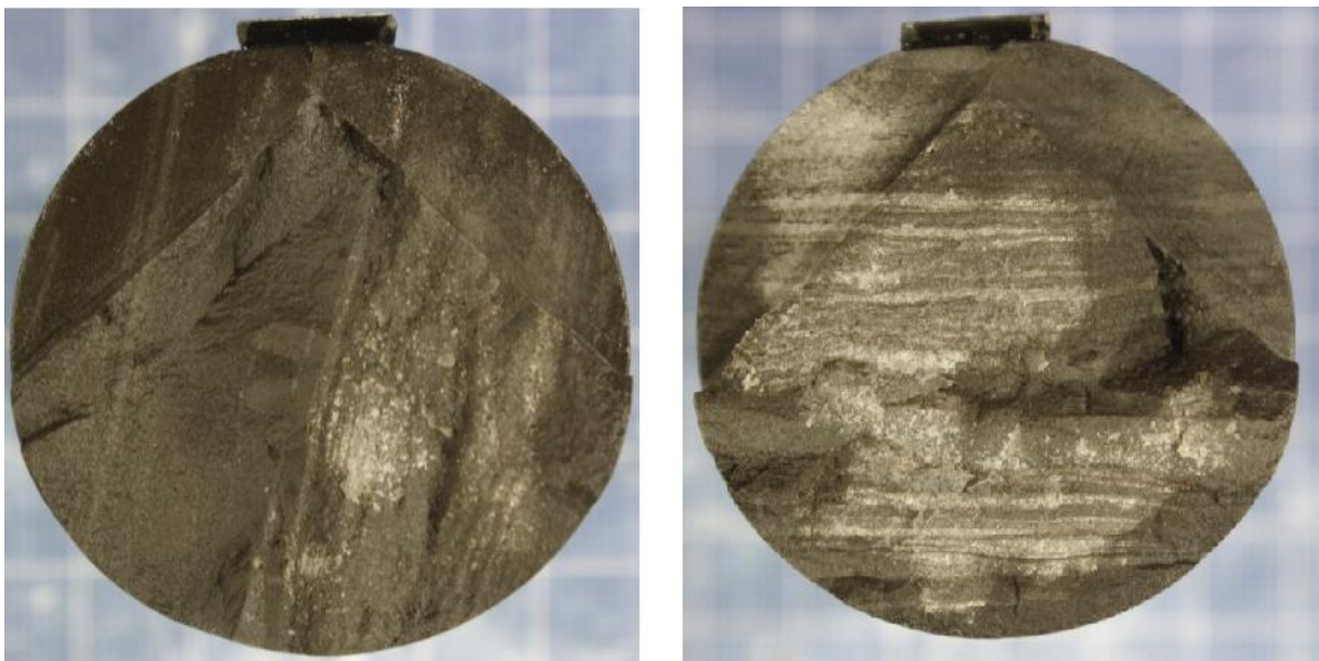
Figure 4-6: The picture to the left show a notch parallel with the bedding planes, the picture to the right shows a notch perpendicular to the bedding planes. Both pictures are of samples with an inclination of 75°
