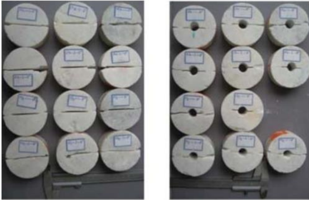
Figure 3-5: Fractured samples from the CCNBD and HCCD experiment. Notice the cracks that have propagated in tensile mode. CCNBD is to the left, HCCD is to the right (Amrollahi & Baghbanan, 2009)
