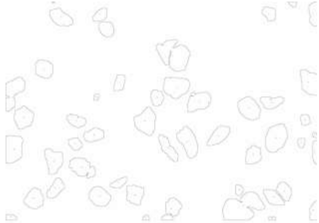
Figure 44 Outlines of the particles from a SEM picture, used for calculating shape descriptors in ImageJ.
