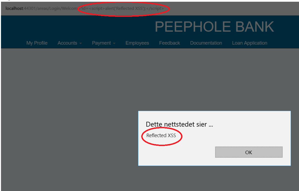
Figure 4.13: Screenshot showing what happens when we change the variable in the URL to a script
