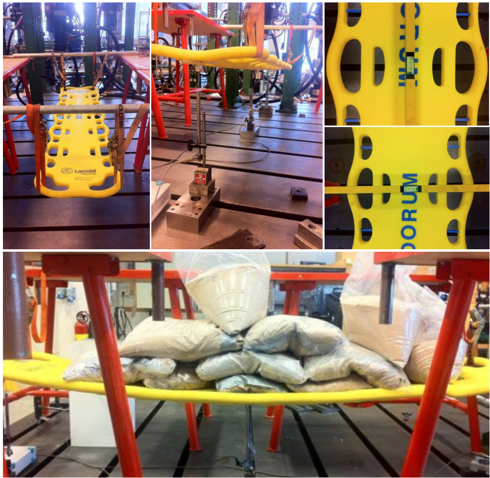
Figure 50: Equipment setup for the bending test
