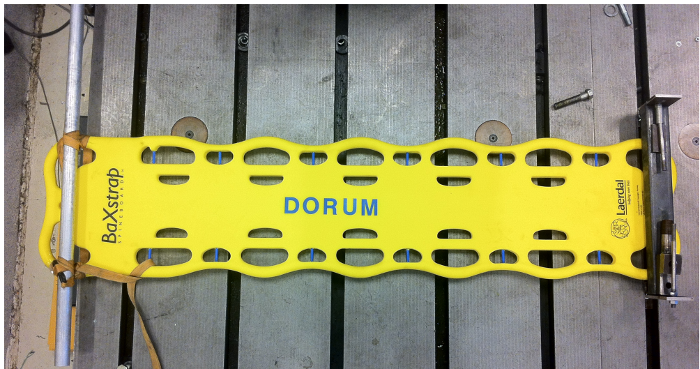
Figure 46: Setup for the torsion test, according to NS-EN 1865:2000
