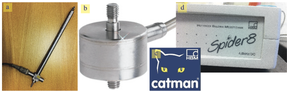
Figure 45: Equipment utilized for load/distance-measurement
