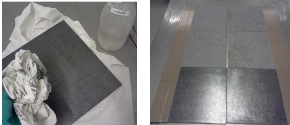
Figure 5: Surface cleaning after needle scaler. Needle scaled surface (bottom) is glossy and dark compared to grit blasted (top).
