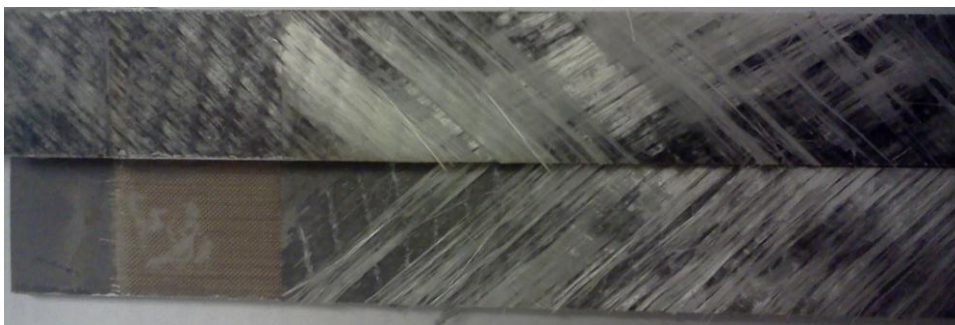
Figure 13 Crack surface DCB-GC-4
