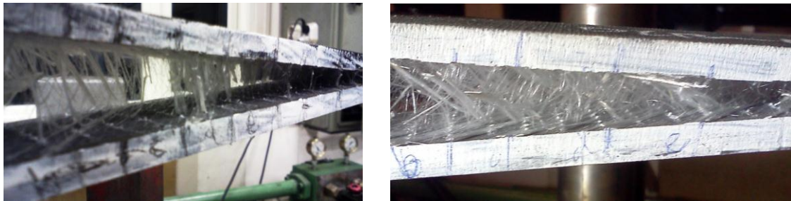
Figure 12 Fibre bridging on DCB-GC-1 (left) and DCB-GC-2 (right)
