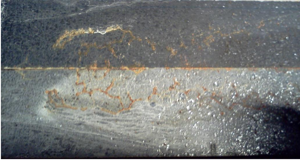
Figure 9 Interface of delaminated ENF-NP specimen.
