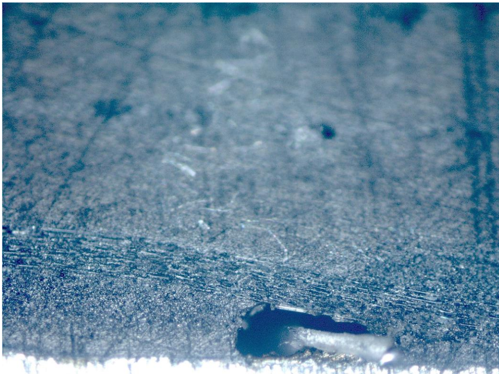
Figure 34: Bondline of ENF-GP5 10x
