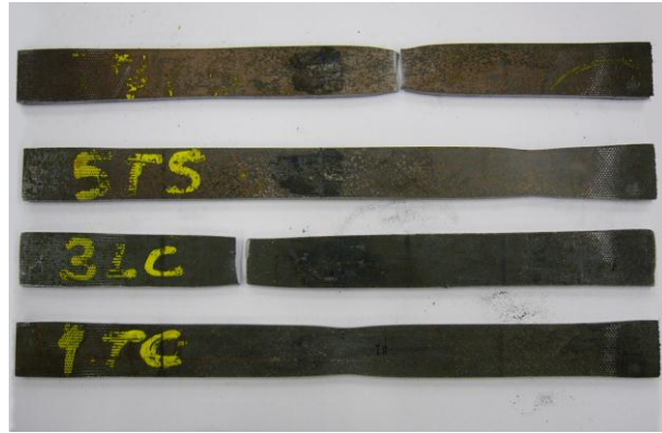
Fig.5: Typical failure modes of selected specimens (1TC, 3LC, 5TS and 7LS).
