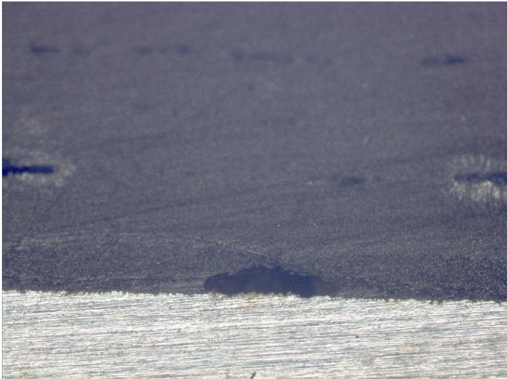
Figure 33: Bondline of ENF-GP5 5x
