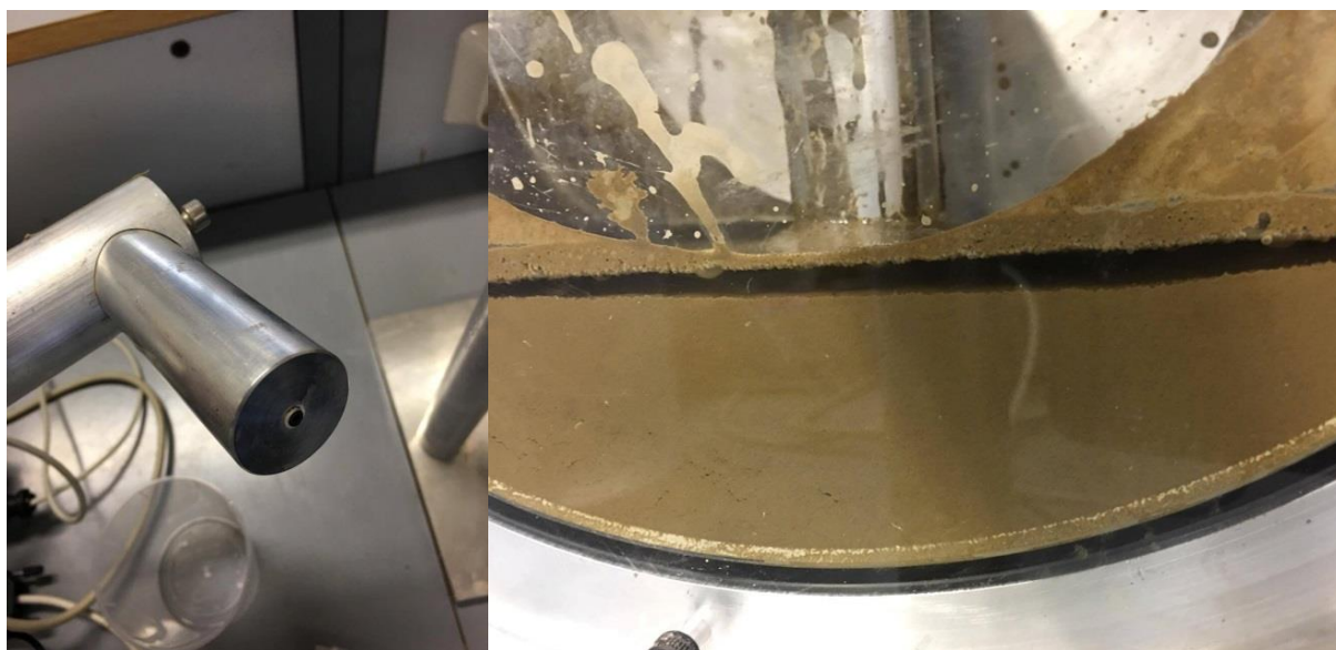
Figure 4-7 The sensor bar and its insertion
