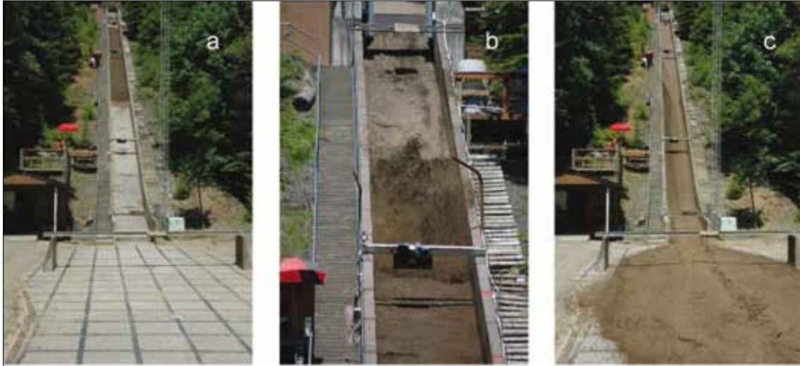
Figure 2-9 Debris flow behavior during a large scale experiment with wet bed sediment (a) Release of the flow (b) Close up of the debris flow entraining bed sediment (c) Debris flow crossing the deposition zone (Reid et al., 2011)
