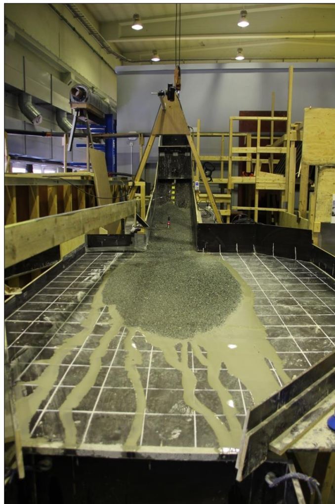
Figure 4-8 Flow deposition in the laboratory experiment (Laache, 2016)
