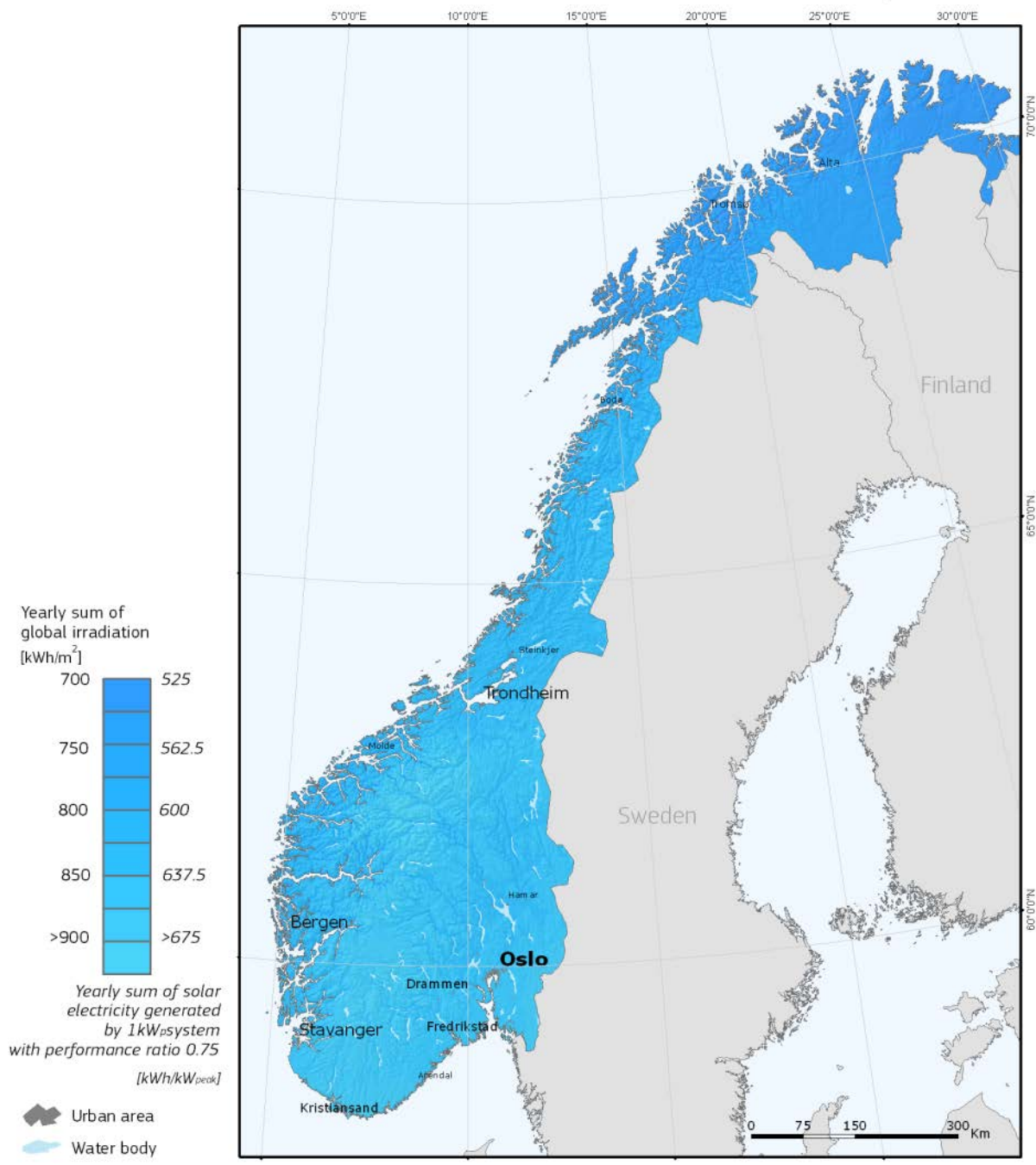
Fig. 1.3. Global irradiation and solar electricity potential in Norway of horizontally-mounted photovoltaics modules (PVGIS 2012).
