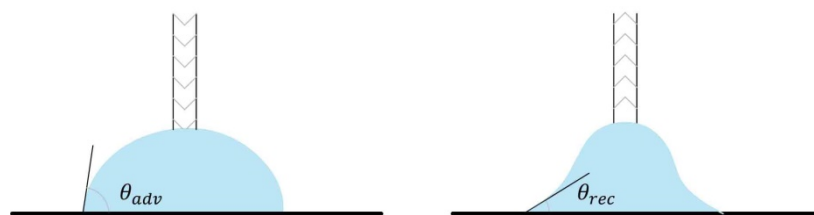
Fig. 4.6. Static drop method to measure the advancing \theta_{adv} (left) and receding \theta_{rec} (right) contact angle of a water droplet on a generic surface.
