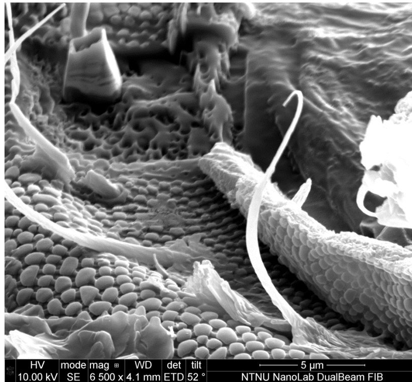
Figure 22 – Sample 1 destroyed by high current
