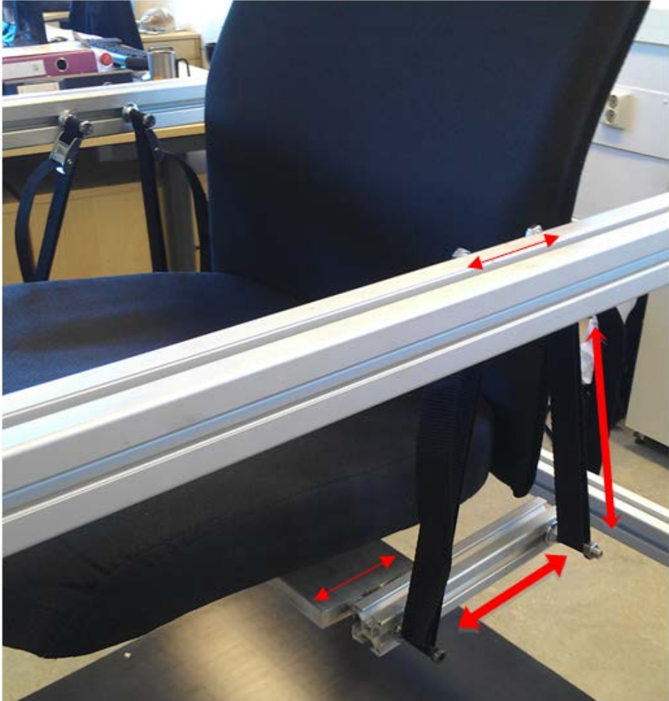
Figure 26: Adjustment possibilities on the test rig
