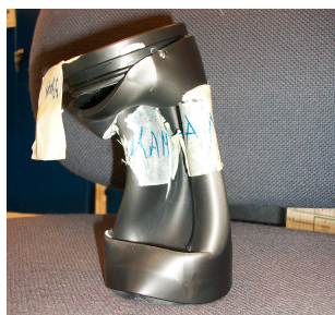
Figur 1.1: Bukla kamerahus i aluminium
