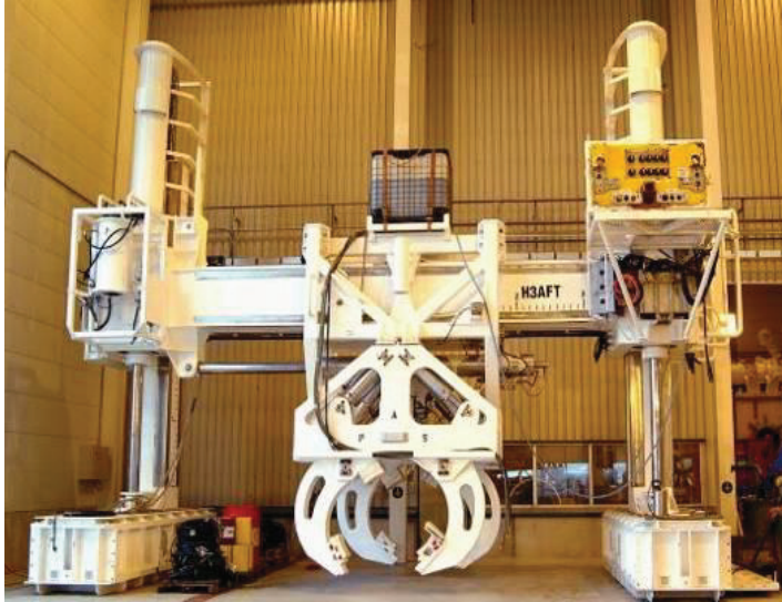
Fig. 2: H-frames for lifting the pipeline after removing the damaged section.
