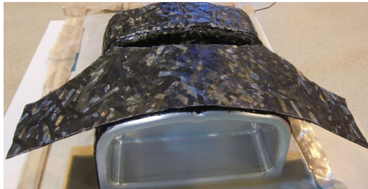
Figure 14: Layup of C-shaped M61 [Photo: Nina Thorvaldsen]
