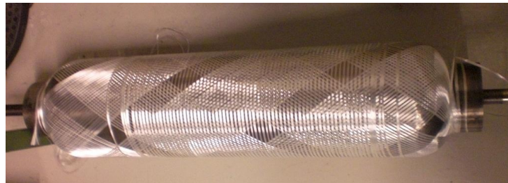
Figure 8: Filament winding test done at NTNU by the polymer and composite group
