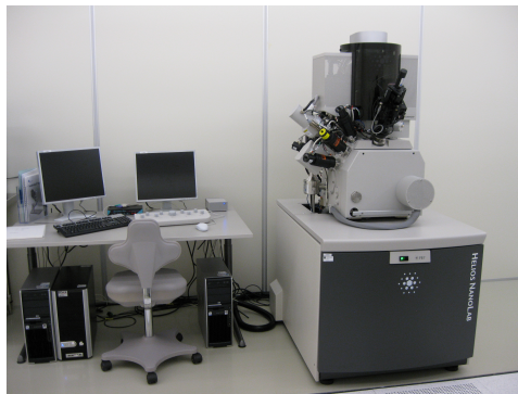
Figure 26: FIB machine with SEM at NTNU Nanolab [29].
