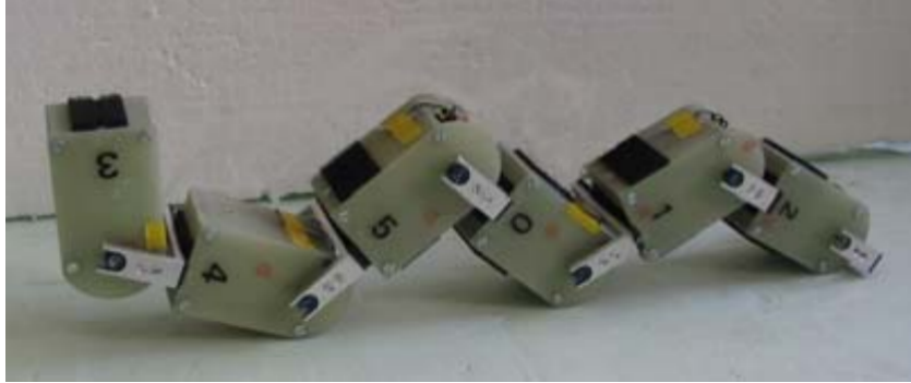
Figure 2.2: Yamor robots configured as a snake[39].
