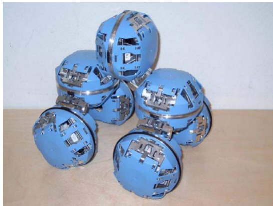
Figure 2.3: Atron assembled into a four wheeled car [9].
