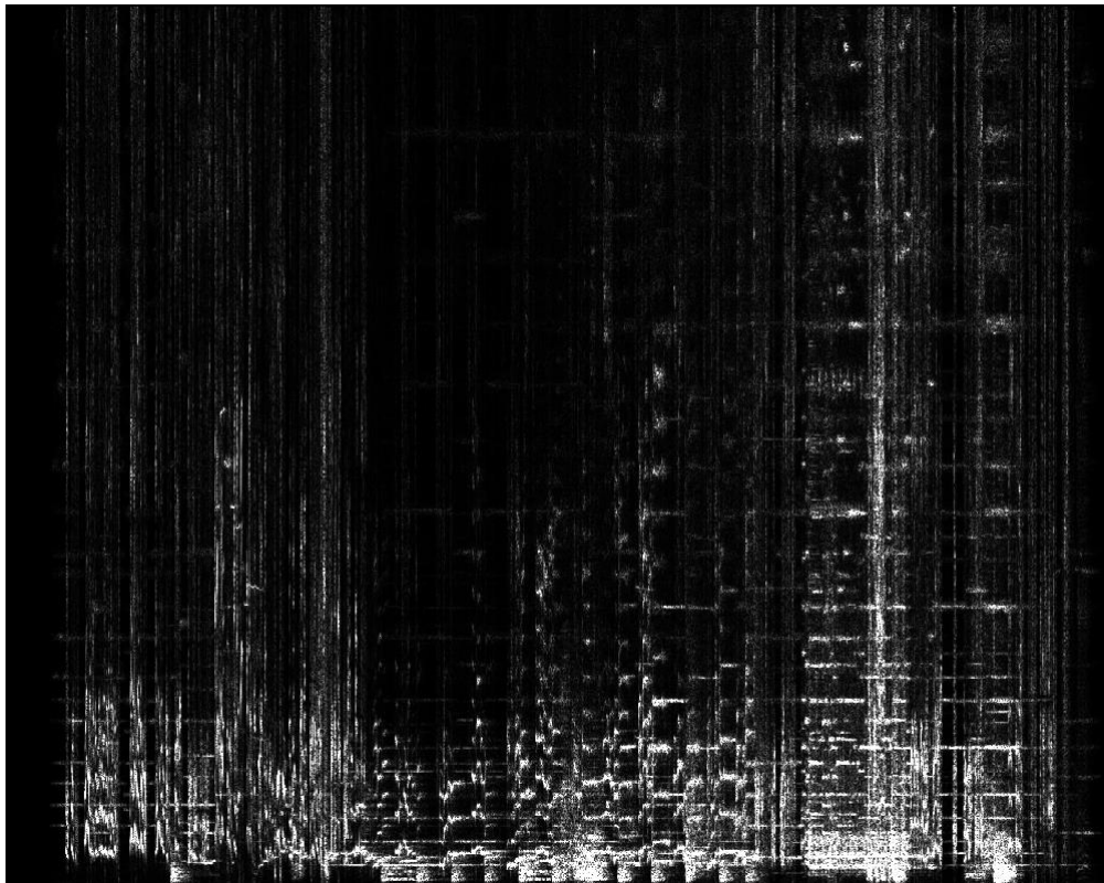
Figure 3.3: Visualization of a frequency spectrogram, generated by the Acoustic Fingerprinting Library.
