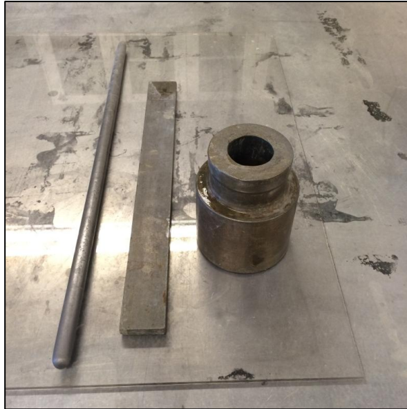
Picture 3 The steel cone, steel rod and steel flat
