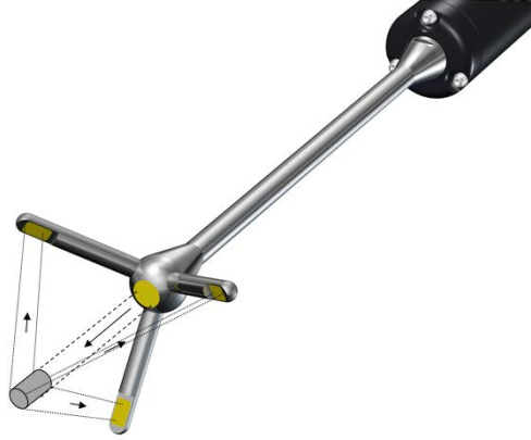
Figure 14 – Principle of operation of a three-branch ADV probe. Acoustic waves are generated by the central emitter, reflected by particles moving in the sampling volume and propagating back to one of the three receivers.
