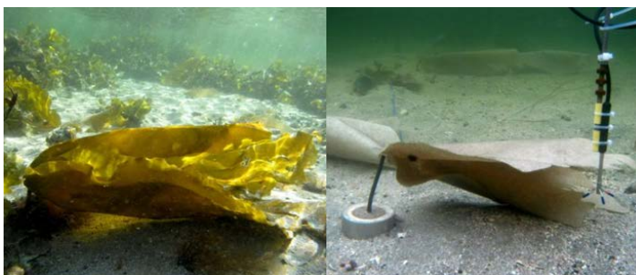
Figure 13 – Implementation of a drag force sensor in the field for testing the hydrodynamic performance of a L. digitata surrogate (right), and comparison with its natural counterpart (unpublished data – PISCES project).
