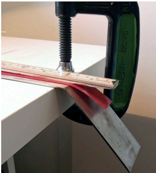
Fig. 2. Picture of the cantilever test device applied to one of the artificial materials (Sample 1).
