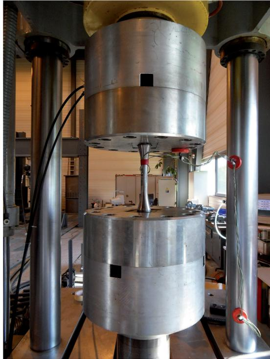
Figure 7: Experimental set-up for fatigue testing of  $\varnothing 21$  specimens.
