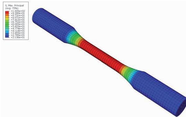
Fig. 2. Stress distribution in Ø16 fatigue specimen.
