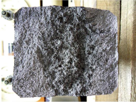
Figure 9: Cross section of a broken 120 mm  $\times$  140 mm specimen.
