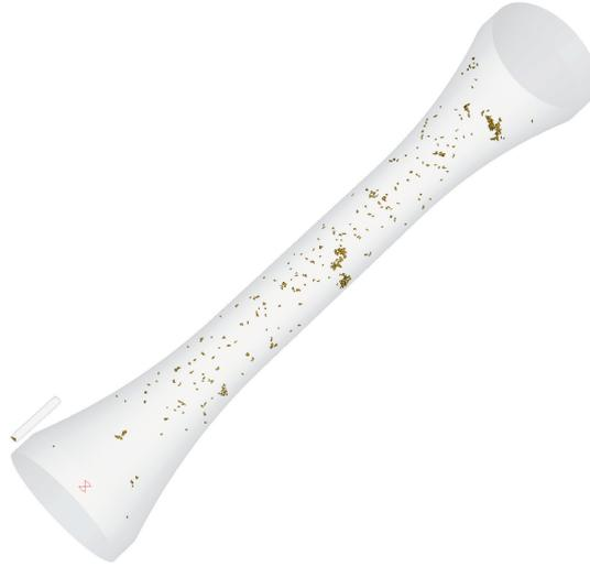
Figure 3.4: Defects detected by 3D X-ray computed tomography (XCT) in a fatigue specimen from a rejected wind turbine hub.
