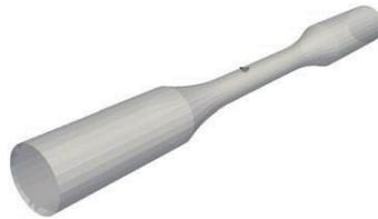
Fig. 3. Defect inserted on the Ø16 fatigue specimen surface.
