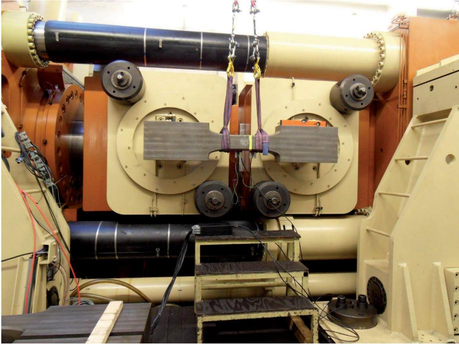
Figure 8: Experimental set-up for fatigue testing of 120 mm × 140 mm specimens.
