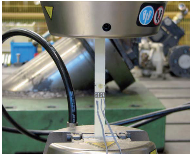
Figure 7-1 Tensile testing of glass fiber specimen at NTNU/SINTEF fatigue laboratory.
