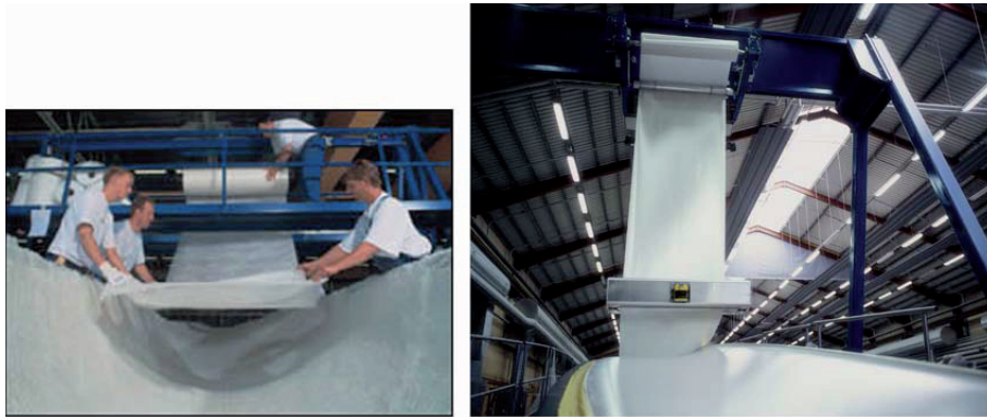
Figure 8-17 Manual and automatic placement of plies for a wind turbine blade at LM Fiberglass (Plastics Technology, 2008).
