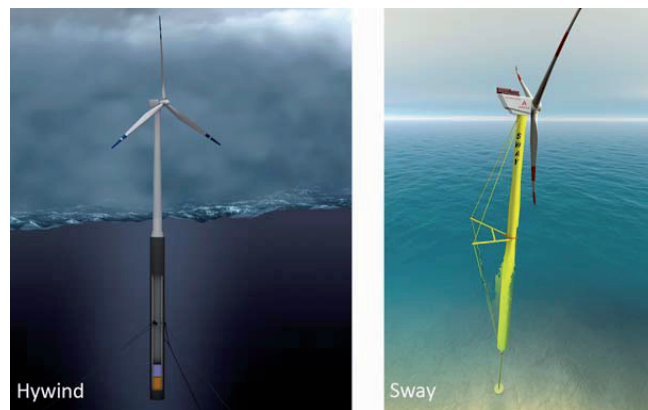
Figure 1-2 Offshore wind turbine concepts by Hywind and Sway.
