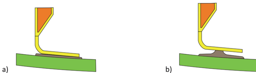
Figure 10-21 a) Ideal bonding of shear web and flange. b) Large gap between parts causing the adhesive to drain away due to insufficient thixotropy.
