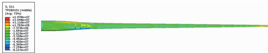
Figure 12-9 Axial stress in top flange \pm 45^\circ ply during 50-year gust.
