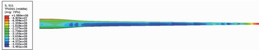
Figure 12-8 Axial stress in top flange UD ply during 50-year gust.
