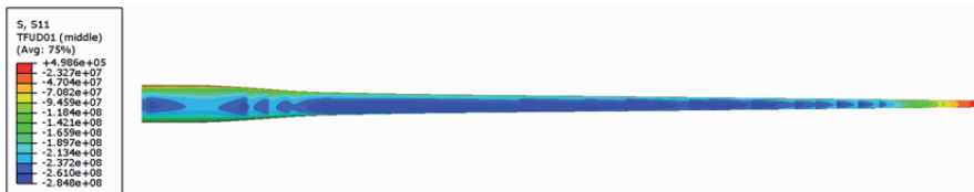
Figure 12-3 Axial stresses in UD glass ply for glass fiber spar with no stiffness criterion.
