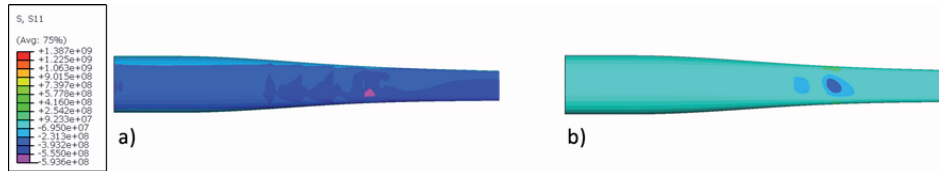
Figure 9-14 Axial stress plots of top flange for a 100 m spar with ply lay-up based on results from compression model. a) UD ply. b) \pm 45^\circ ply.
