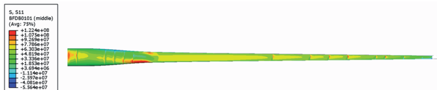
Figure 12-15 Axial stress in bottom flange \pm 45^\circ ply during 50-year gust.
