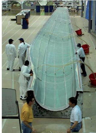
Figure 6-7 Resin infusion of wind turbine blade (www.stanford.edu)
