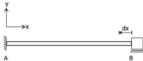
Figure 9-6 Boundary conditions of compression model.
