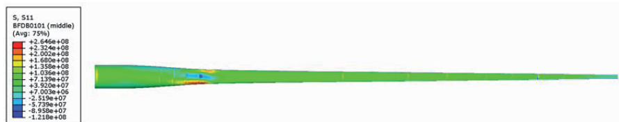
Figure 12-7 Axial stress in bottom flange \pm 45^\circ ply during 50-year gust.
