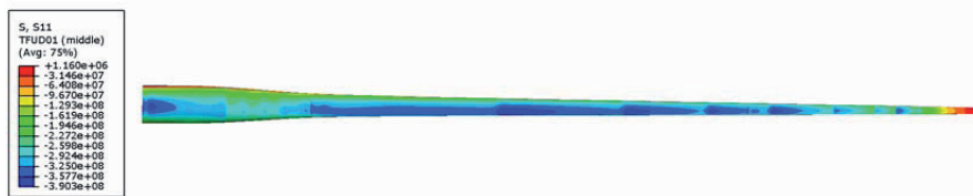
Figure 12-2 Axial stresses in UD carbon ply for carbon fiber spar with stiffness criterion.
