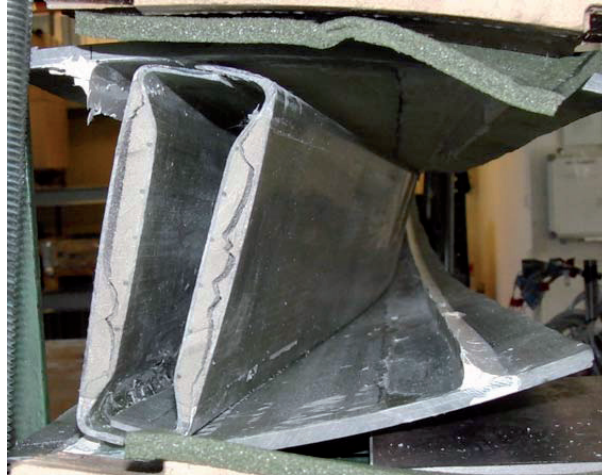
Figure 10-22 Failure of bond between shear web and flange at the left side of the spar.
