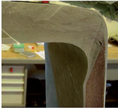
Figure 10-3 Tapering of core material in shear web of wind turbine spar (reproduced from F. M. Jensen et al., 2006).
