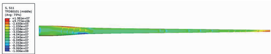
Figure 12-13 Axial stress in top flange \pm 45^\circ ply during 50-year gust.
