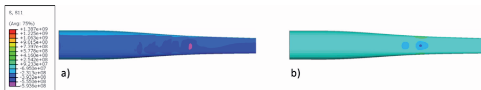
Figure 9-13 Axial stress plots of top flange for a 100 m spar with ply lay-up based on results from bending model. a) UD ply. b) \pm 45^\circ ply.
