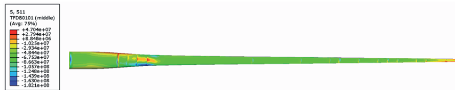
Figure 12-5 Axial stress in top flange \pm 45^\circ ply during 50-year gust.
