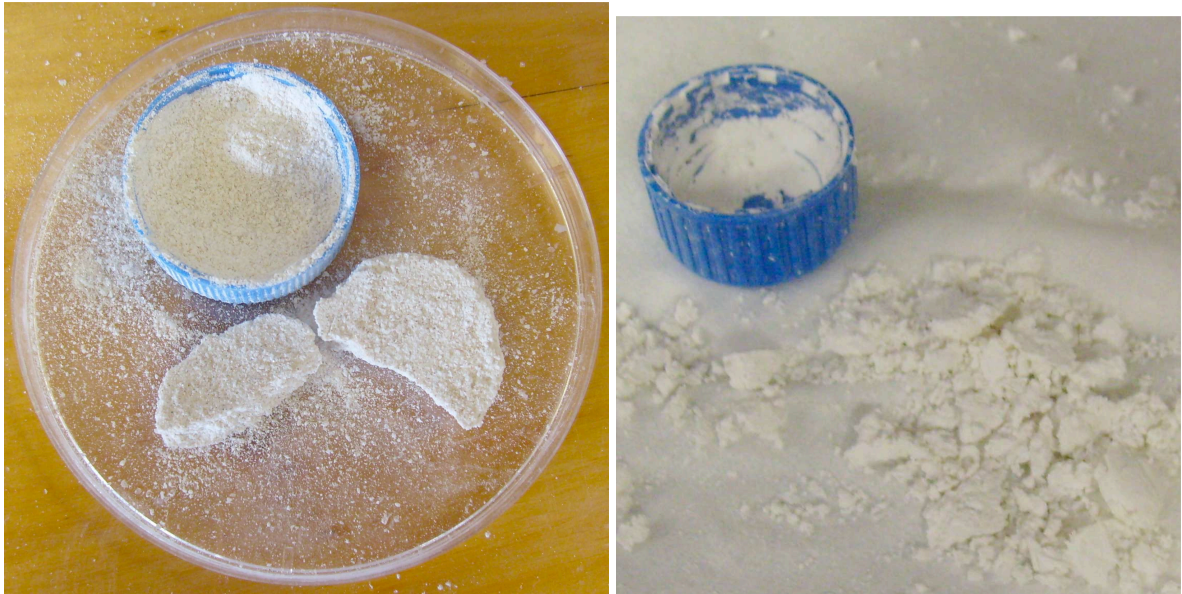
Figure 15. Picture from small-scale test with the improved material mixture to the left and from the small-scale testing with the first recipe (see Table 4 and 5) to the right.
