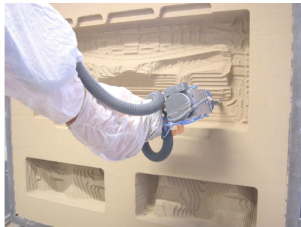
Figure 4. The ConiferRob® technique in progress [9].
