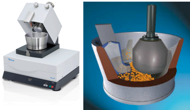
Figure 8. The mechanism of the Retsch RM 200 Mortar Grinder [12].
