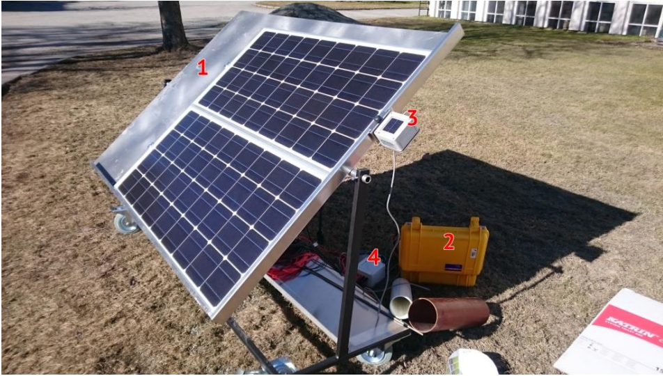
Figure 4.1: Experimental setup for outdoor experiments. 1. Mechanical rig, 2. PVPM measuring device, 3. Irradiance/temperature sensor, 4. Connection between PV modules and PVPM through a safety switch. (Photo: Lovinda Ødegården)
