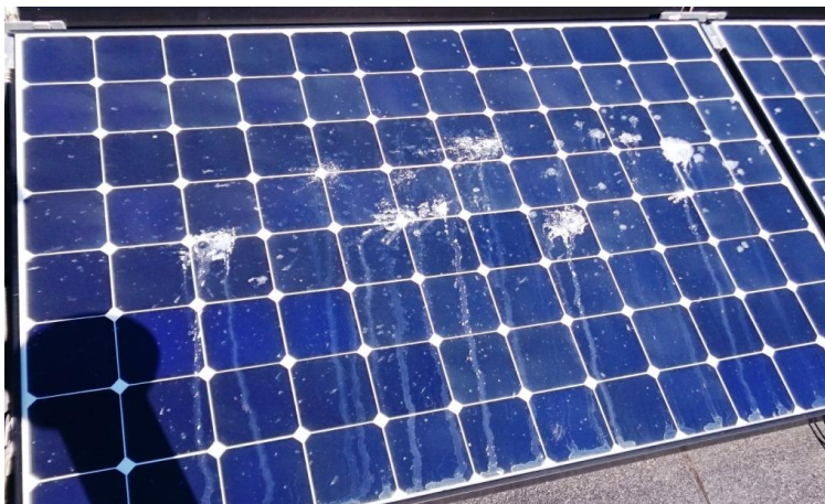
Figure 2.11: A module severely soiled by seagull droppings in addition to partial shading, taken 10:30 March 10th. (Photo by L. Ødegården)
