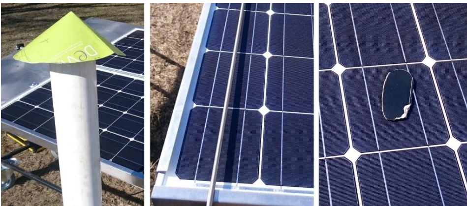
Figure 4.3: The three recreations of shading at PK: The vent pipe (left), safety wire (middle) and blue mussel shell (right). (Photos: Lovinda Ødegården)
