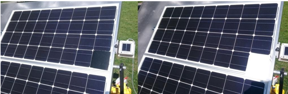
Figure 4.2: Setup for the test measurements on the SoloSol modules. (Photo: Lovinda Ødegården)
