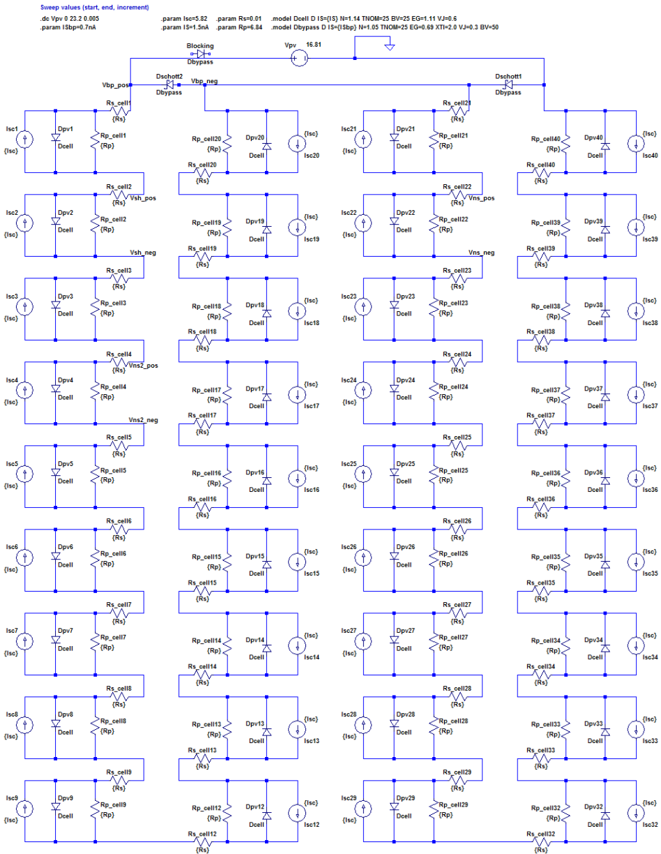
Figure C.2: The LTSpice model for the IBC SoloSol 100 CS module. The blocking diode is not connected.
