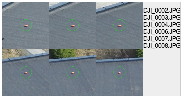
Figure 7: Images in which GCPs have been marked (yellow circle) and in which their computed 3D points have been projected (green circle). A green circle outside of the yellow circle indicates either an accuracy issue or a GCP issue.
