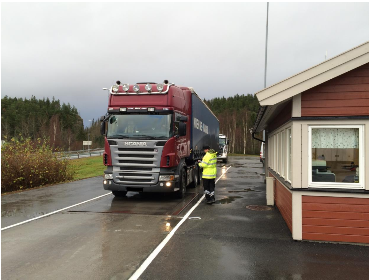
Figure 15: A photo showing the static plate weight at the traffic station, measuring the front axle of a vehicle. Photo: Torbjørn Haugen.
