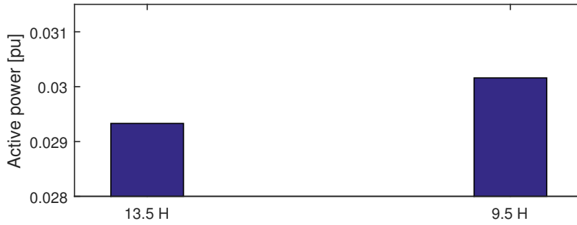
Figure C.8: Total loss from the wind turbines to the grid for the systems operating with different shunt reactors. The legend shows the inductance value used in the shunt reactors.
