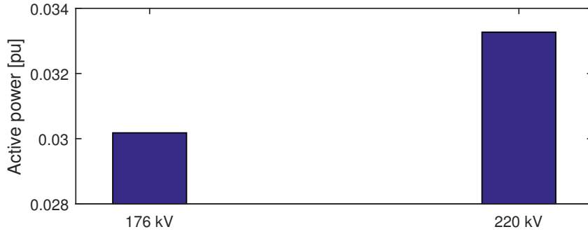
Figure C.6: Total loss from the wind turbines to the grid for the systems with different transmission voltage level at constant wind speed.
