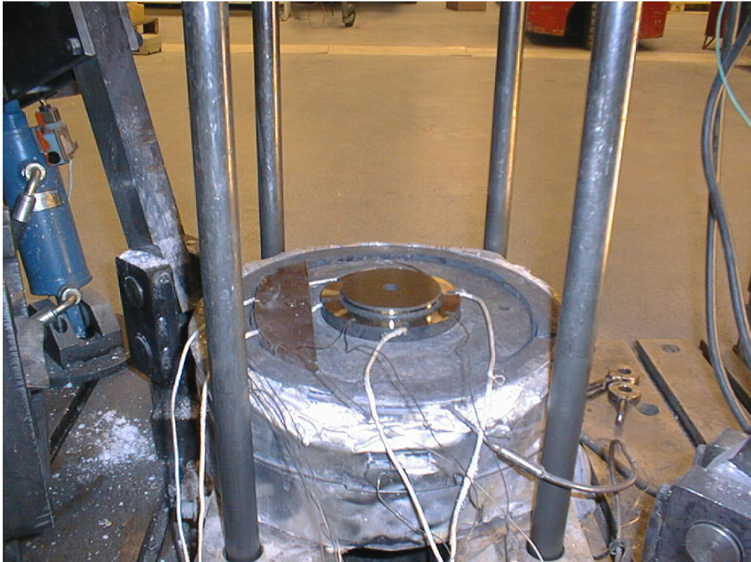
Figure 2.3. An extrusion die mounted in the container. The die is instrumented, but is not of the complex kind described in the current report.
