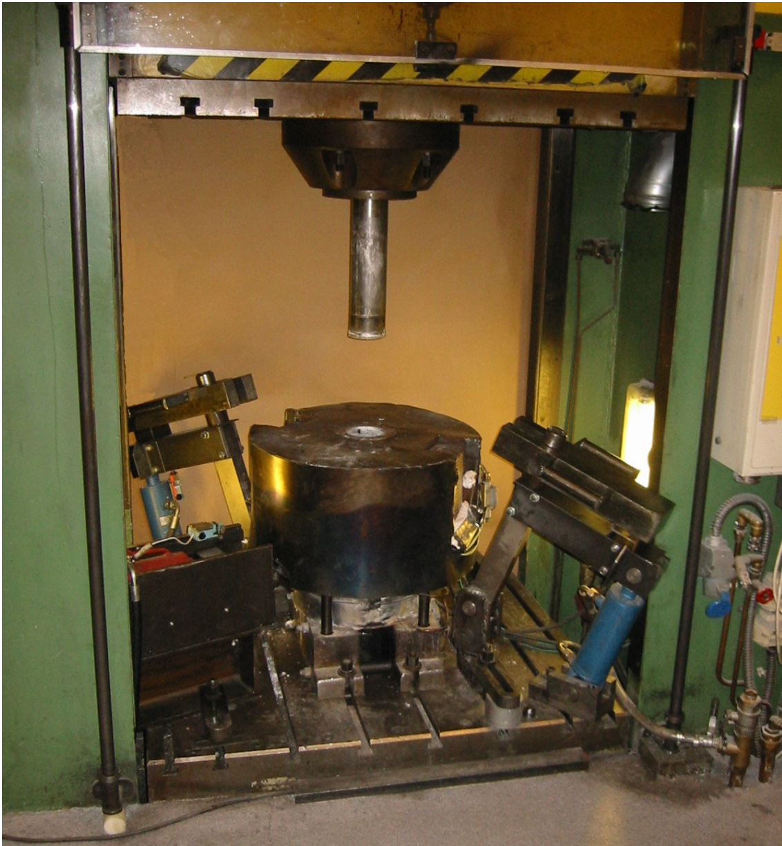
Figure 2.1. The SINTEF 8 MN vertical laboratory press in Trondheim, Norway. The diameter of the ram and container bore is approximately 100 mm. The container and tool support rest on the lower press board. The equipment may be dismantled to allow other kinds of experiments (such as forging).
