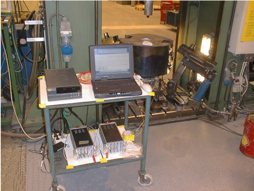
Figure 2.33. The SINTEF extrusion press and the die face and liner load pressure measurement system. The logger was at the left side at the top of the table while the amplifiers were placed on the shelf below the table.
