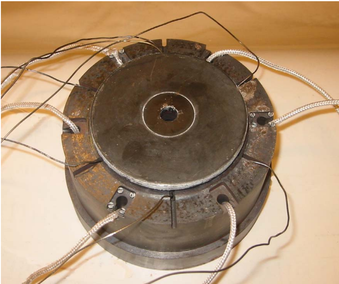
Figure 2.4. A view of the upper face of the complex rod extrusion die. An insert with outlet diameter 11.2 mm ( ER = 80 ) has been used.
