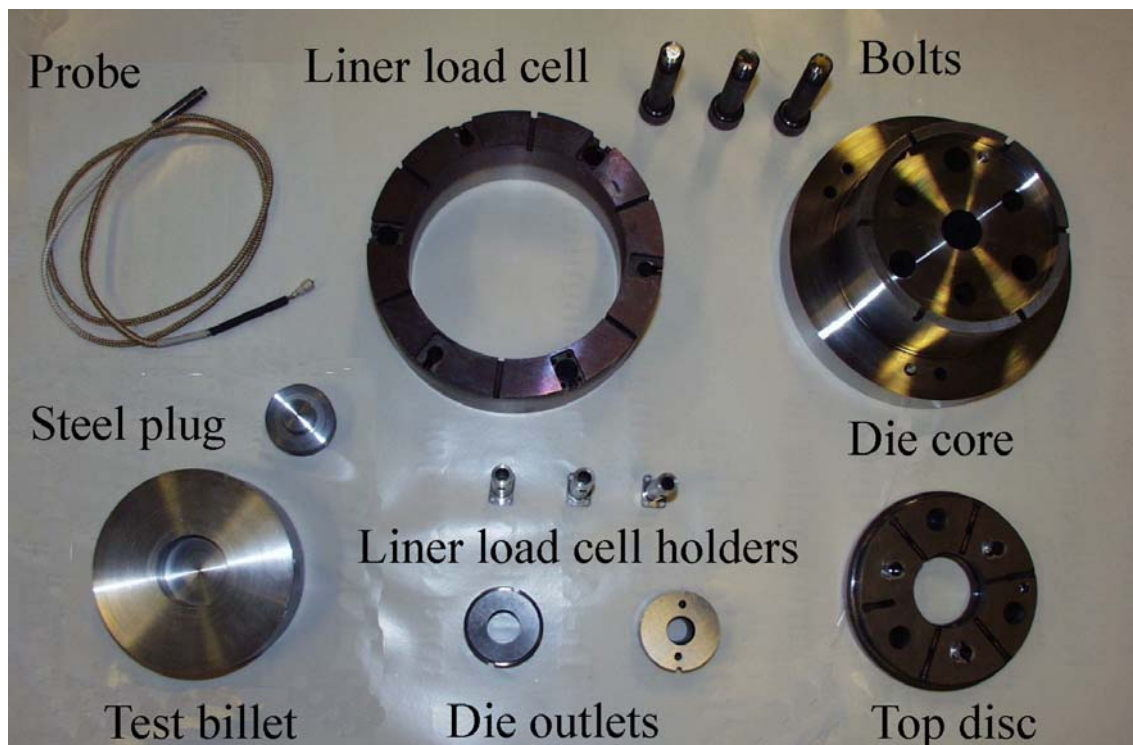
Figure 4.22. The parts of the extrusion and calibration set-up. The test billet and the steel plug are shown on the left hand side.
