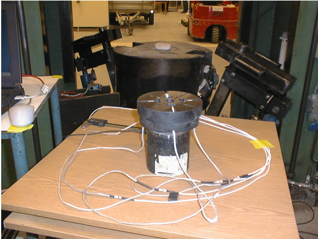
Figure 2.31. The mounting of the capacitive probes (simple die).
