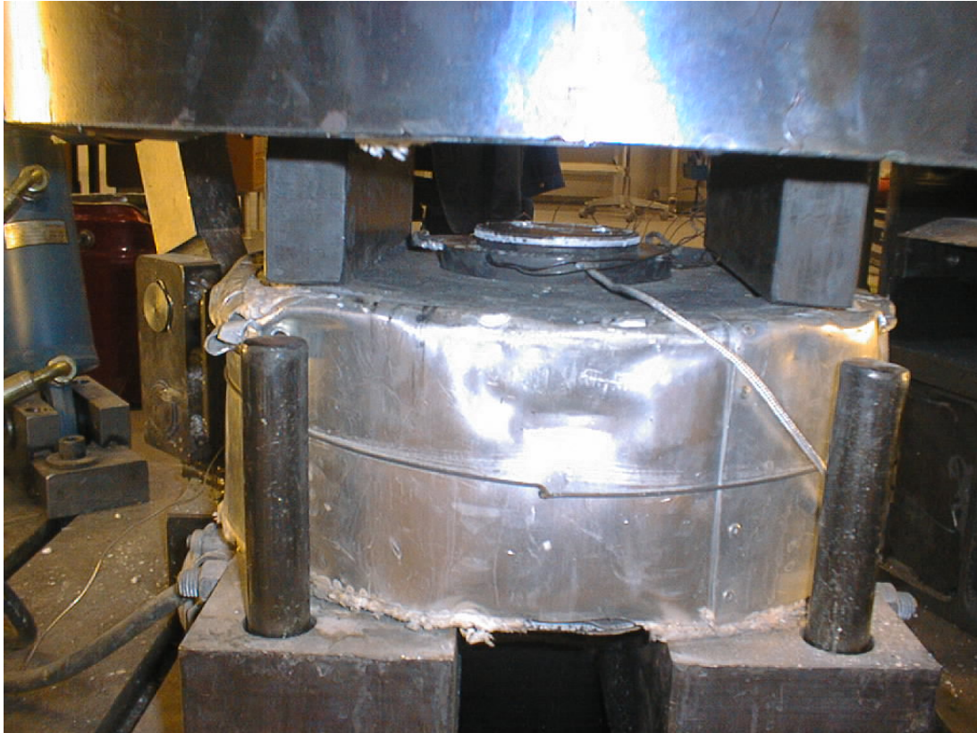
Figure 2.32. The extrusion die (simple type) was placed in the press and the various cables were guided out of the assembly between the bolster and container.
