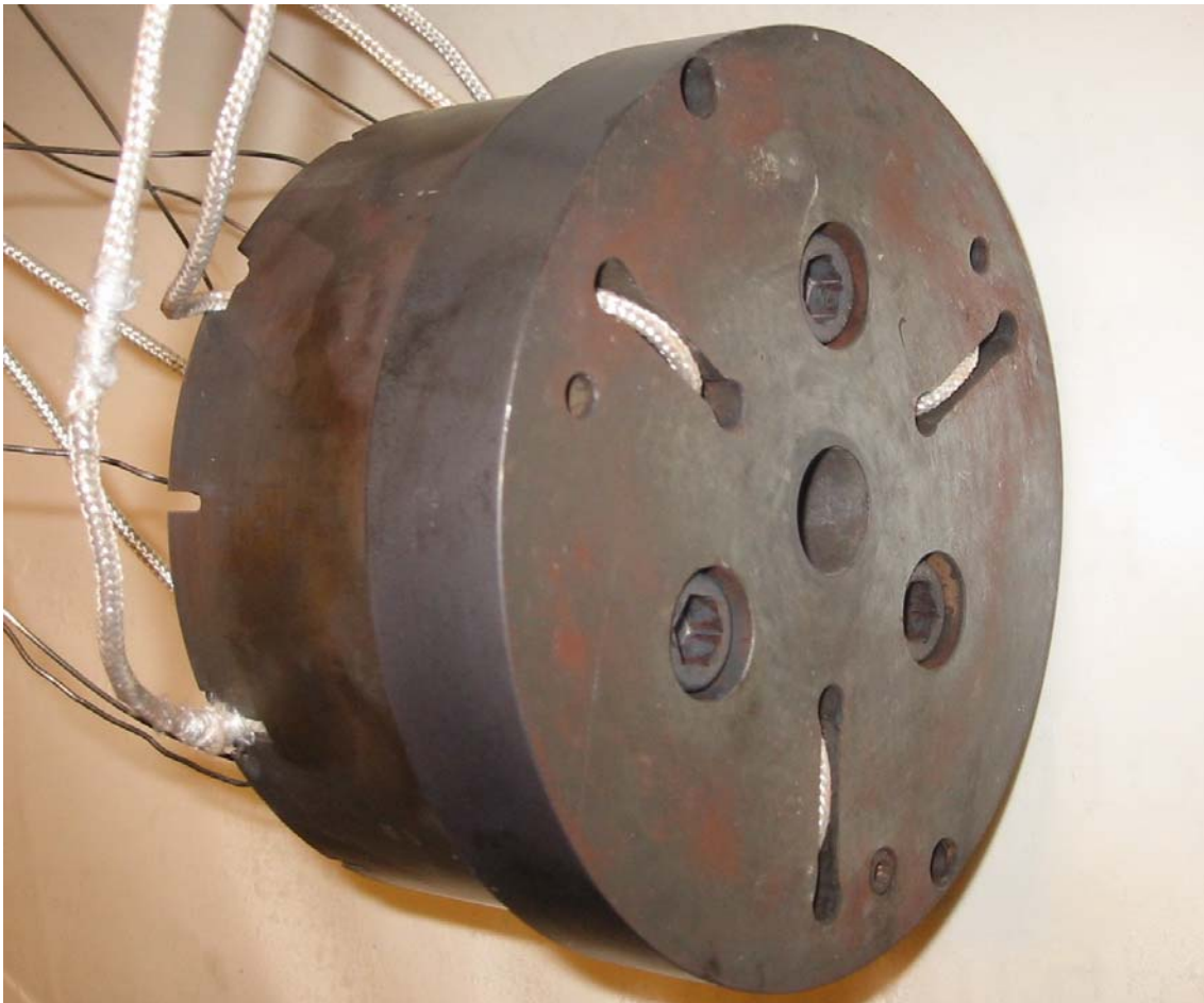
Figure 2.7. A view of the bottom face of the complex rod extrusion die.
