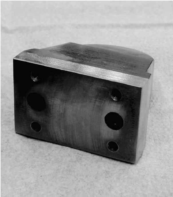
Figure 8 Machined insert, with conformal cooling, used in the modular tool
