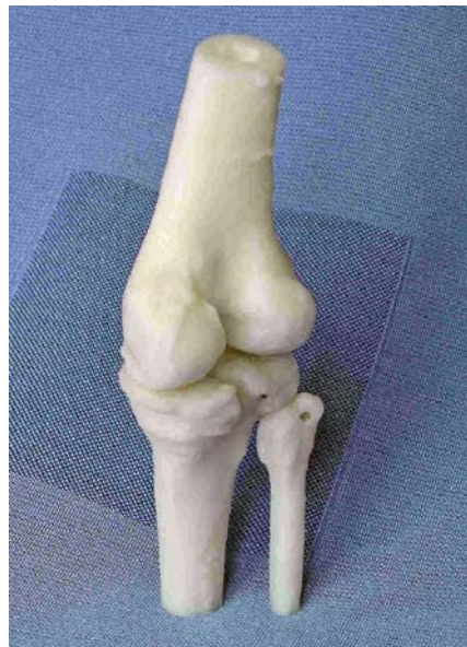
Figure 22. The figure shows a physical model of a knee, where the 3D computer model was obtained from a set of images acquired by a CT scan.
