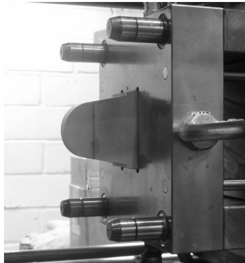
Fig. 4 The core plate with the MD2 insert.
