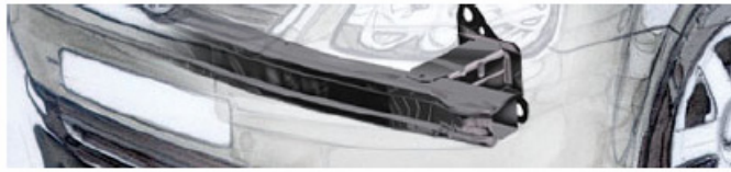
Figure 1: Bumper system consisting of a beam, two crash boxes and a tow nut.
