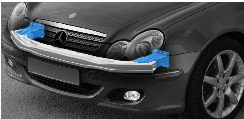
Figure 1.1: Hydro bumper system consisting of a beam, two crash boxes and a tow nut. The crash boxes are highlighted here in blue.
