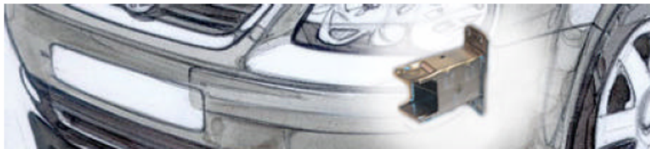
Figure 2: Crash box and its position in the car, behind the bumper on each side (illustration only)
